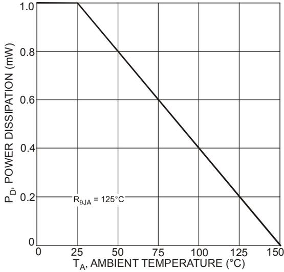
Fig. 1 Power Dissipation vs. Ambient Temperature (Note 4)
