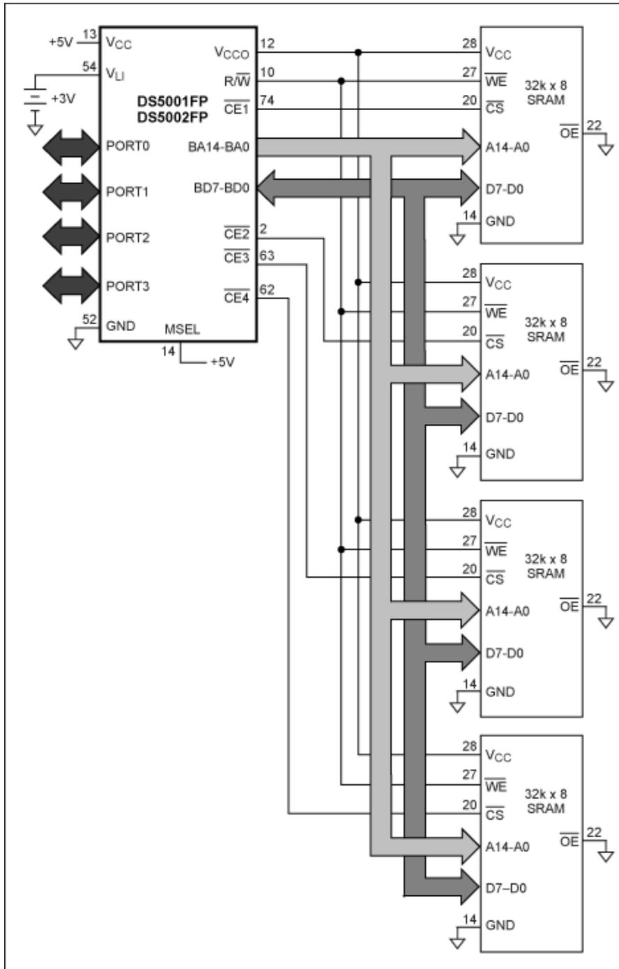
Figure 1. In the multiple-chip memory configuration, external program and data memory are split across four 32kB x 8 SRAM devices.
