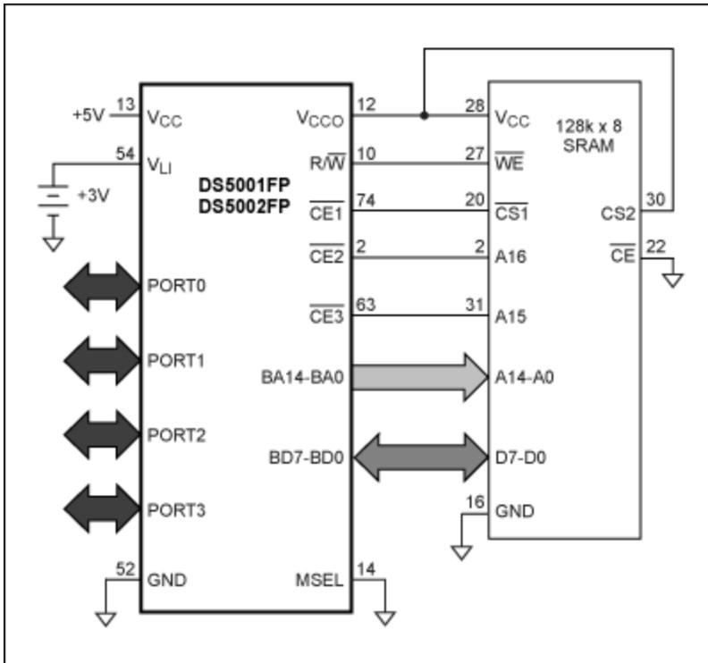
Figure 2. In the single-chip memory configuration, one 128kB x 8 SRAM device holds external program and data memory.
