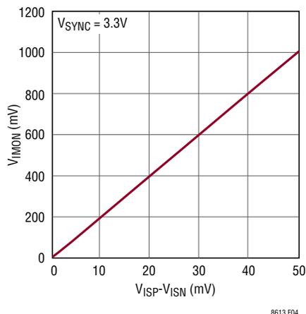
Figure 4. LT8613 Sense Voltage vs IMON Voltage
