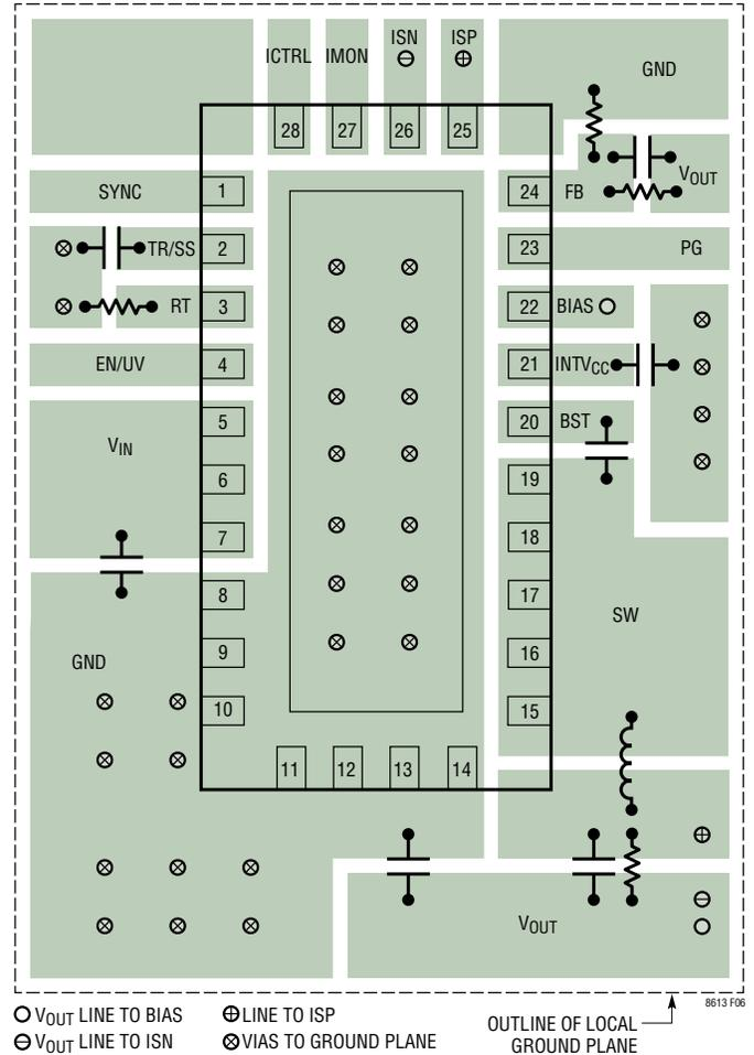
Figure 6. Recommended PCB Layout for the LT8613
