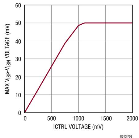
Figure 3. LT8613 Sense Voltage vs ICTRL Voltage
