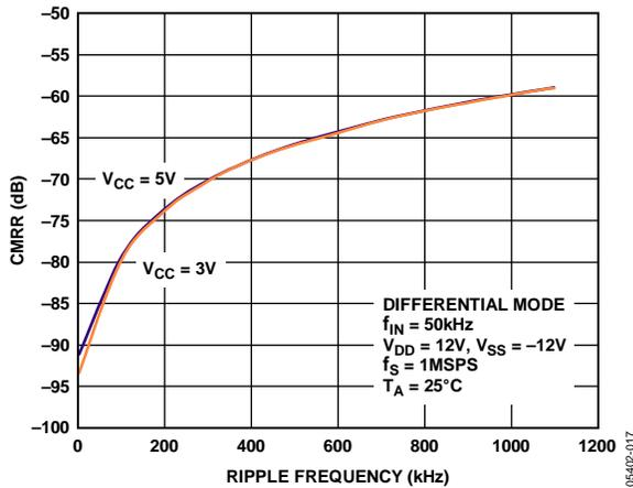
Figure 17. CMRR vs. Common-Mode Ripple Frequency
