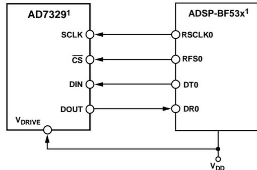
Figure 59. Interfacing the [AD7329](#) to the [ADSP-BF53x](#)
