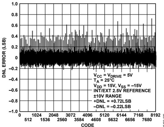
Figure 6. Typical DNL for True Differential Mode
