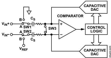
Figure 26. ADC Configuration During Acquisition Phase, Differential Mode
