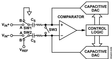
Figure 27. ADC Configuration During Conversion Phase, Differential Mode
