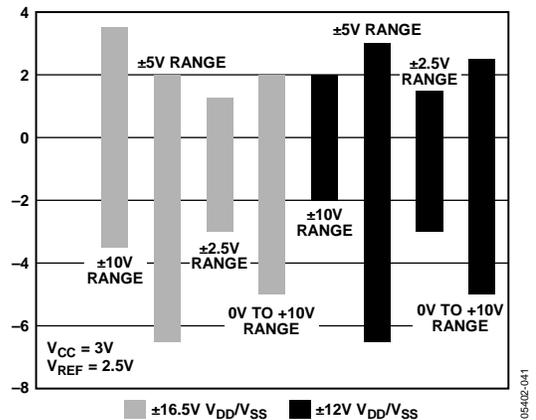
Figure 44. Pseudo Differential Input Range with  $V_{CC} = 3$  V
