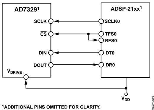
Figure 58. Interfacing the [AD7329](#) to the [ADSP-21xx](#)
