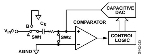
Figure 24. ADC Configuration During Acquisition Phase, Single-Ended Mode
