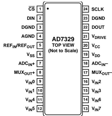
Figure 3. Pin Configuration
