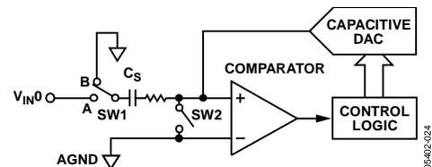
Figure 25. ADC Configuration During Conversion Phase, Single-Ended Mode
