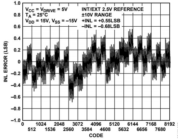
Figure 7. Typical INL for True Differential Mode
