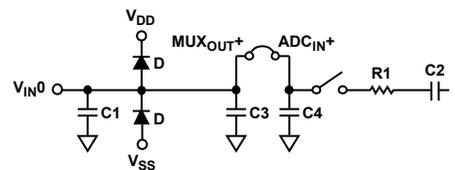
Figure 30. Equivalent Analog Input Circuit, Single-Ended Mode
