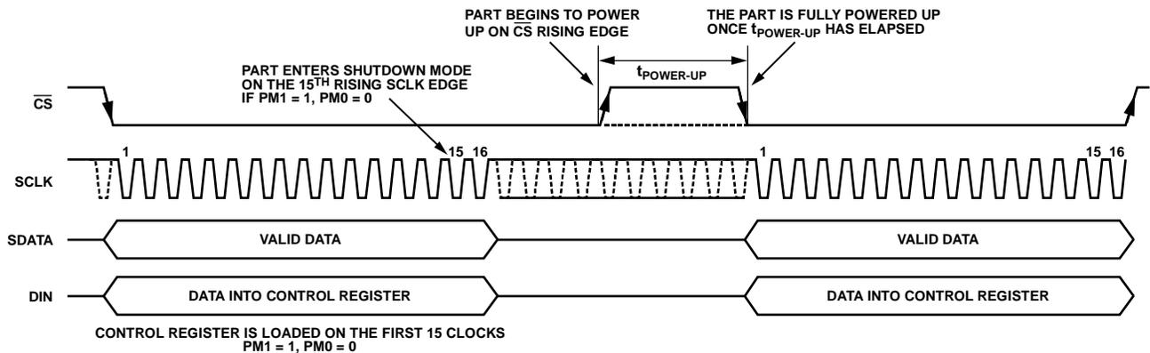
Figure 54. Entering Autoshutdown/Autostandby Mode
