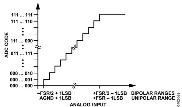
Figure 29. Straight Binary Transfer Characteristic, Bipolar Ranges
