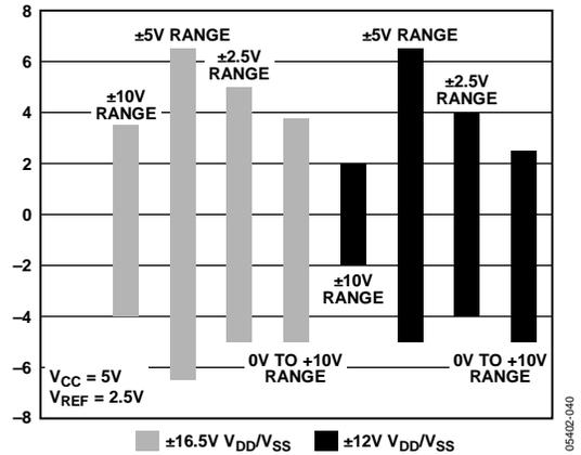
Figure 43. Pseudo Differential Input Range with  $V_{CC} = 5$  V
