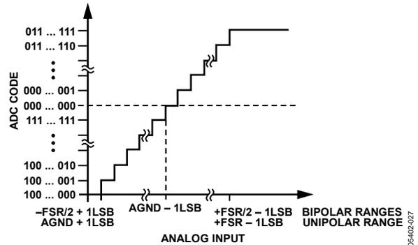
Figure 28. Twos Complement Transfer Characteristic, Bipolar Ranges
