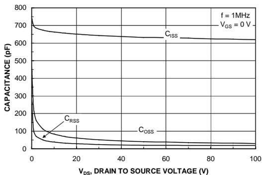
Figure 8. Capacitance Characteristics.
