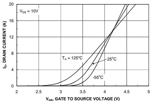
Figure 5. Transfer Characteristics.
