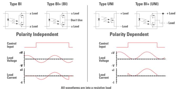
**Type BI** relays conduct load current in both directions.
