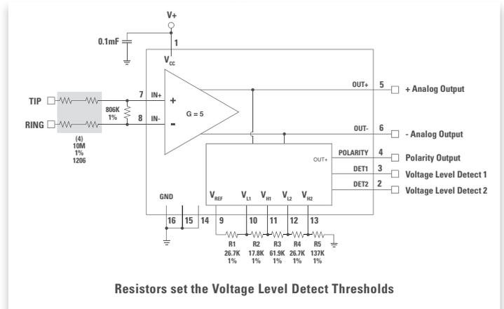
Resistors set the Voltage Level Detect Thresholds
