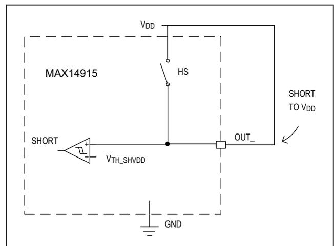
Figure 6. Short to V<sub>DD</sub> Detection Scheme
