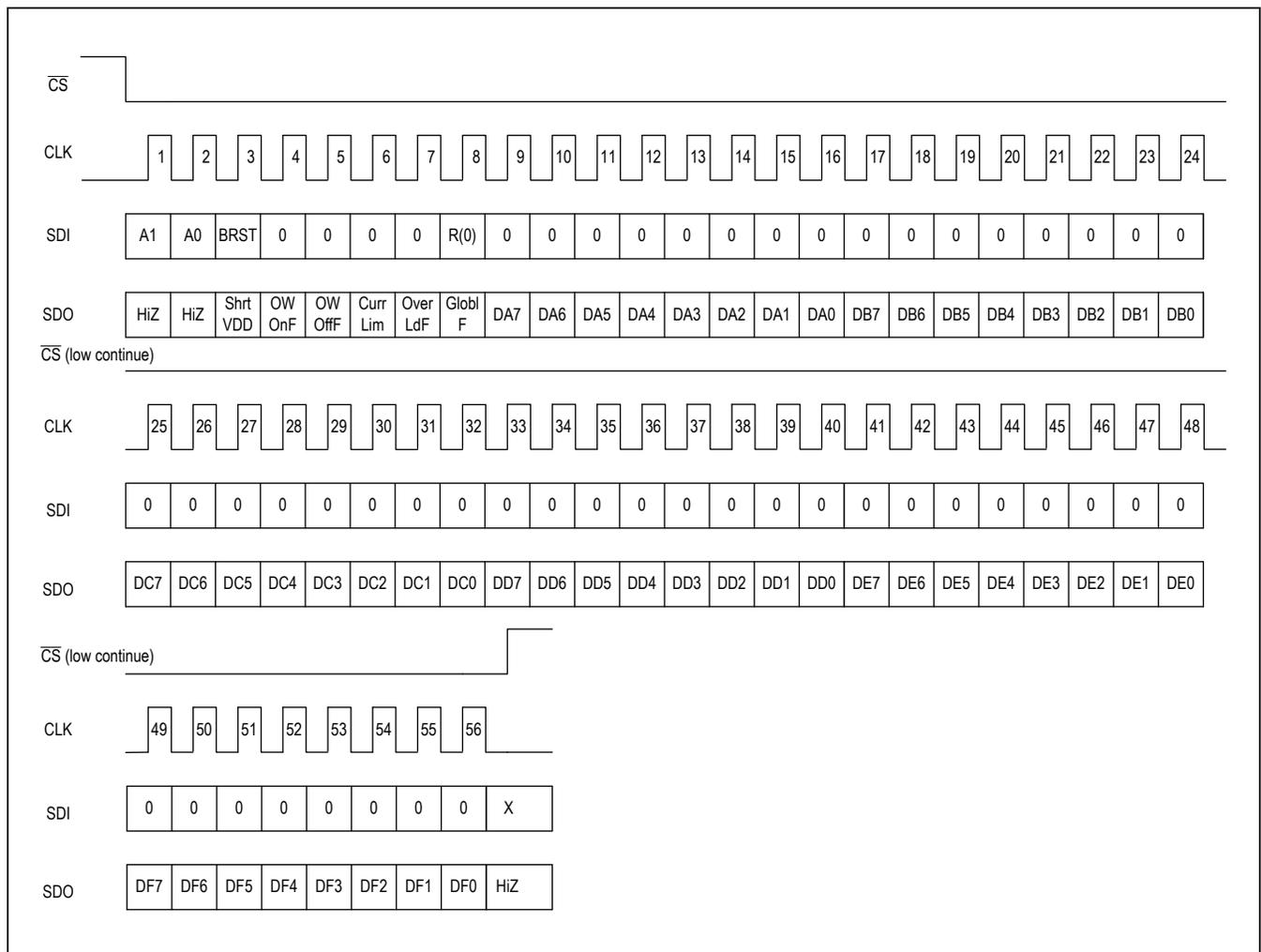
Figure 15. Addressed SPI Six Bytes Burst Read Command
