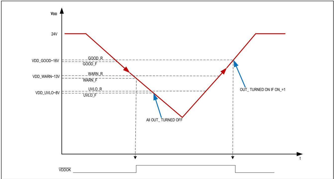
Figure 4.  $V_{DD}$  Monitoring with  $VDDOnThr = 1$
