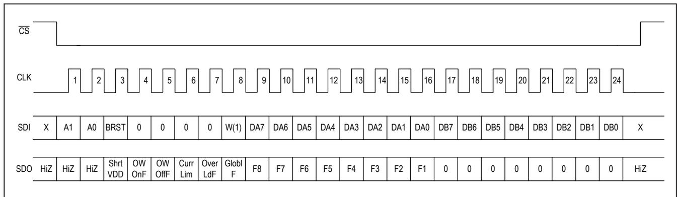
Figure 12. Addressed SPI Single Cycle Write Command
