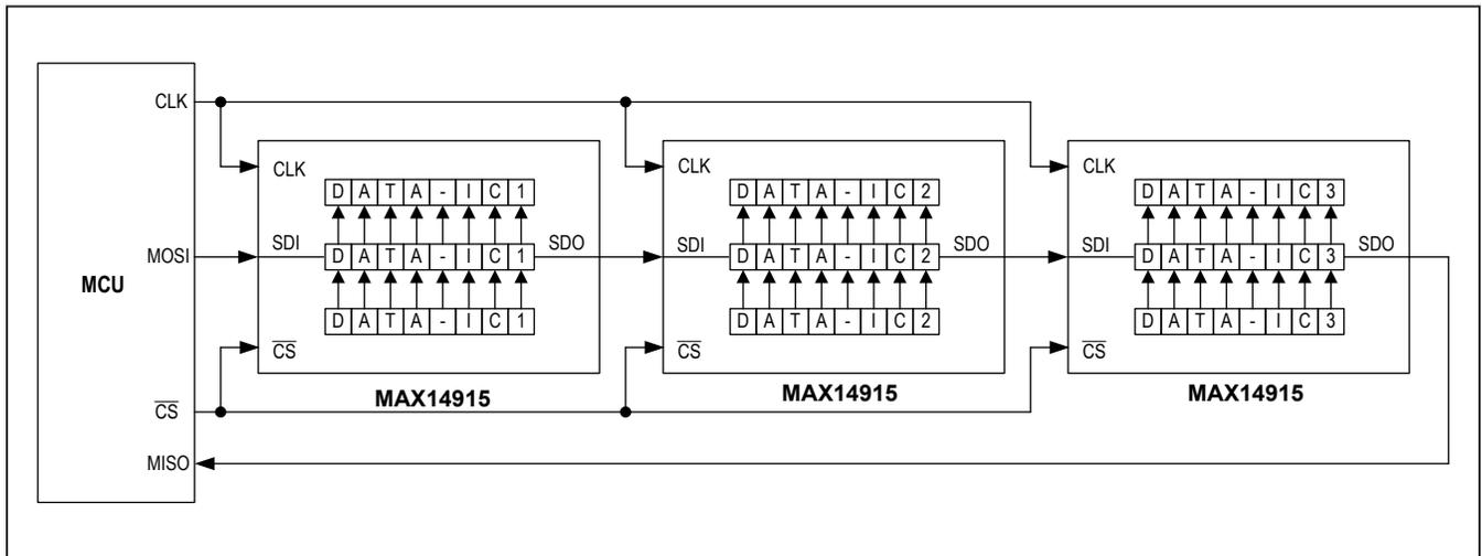
Figure 17. Daisy-Chaining Diagram of Three MAX14915
