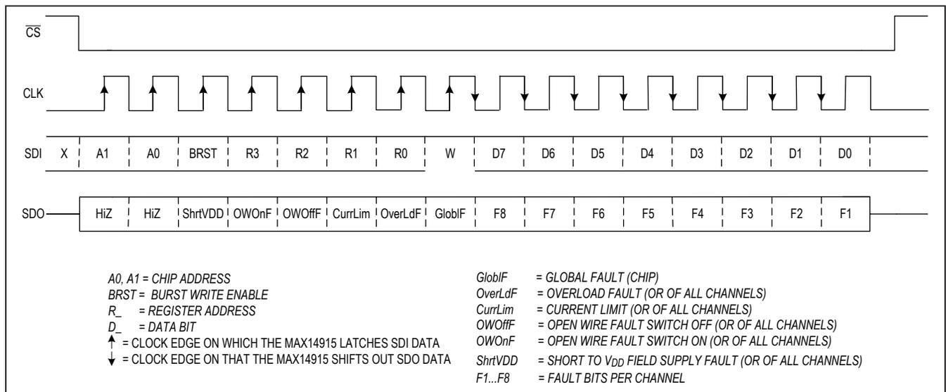
Figure 11. Addressed SPI Single Cycle Write Command
