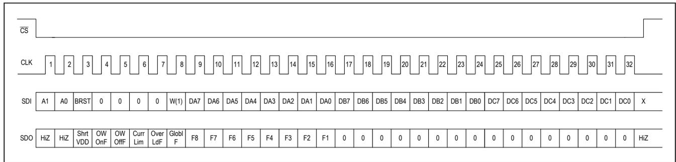
Figure 13. Addressed SPI Three Bytes Burst Write Command
