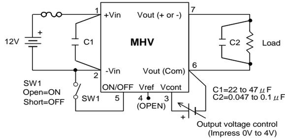
When lowering the output noise even more, keep in mind the input/output wiring, creepage and area distance, while keeping the wiring as thin as possible and layout the C2 near the Load.
