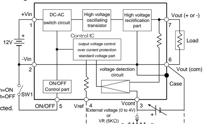
Warning 1: The input-output ground line and case are internally connected.
