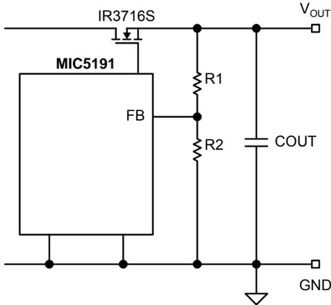
**Figure 10. Adjustable Output**
