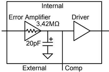
**Figure 3. Internal Compensation**
