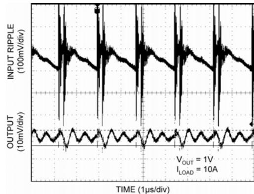
**Figure 11. Ripple Reduction**
