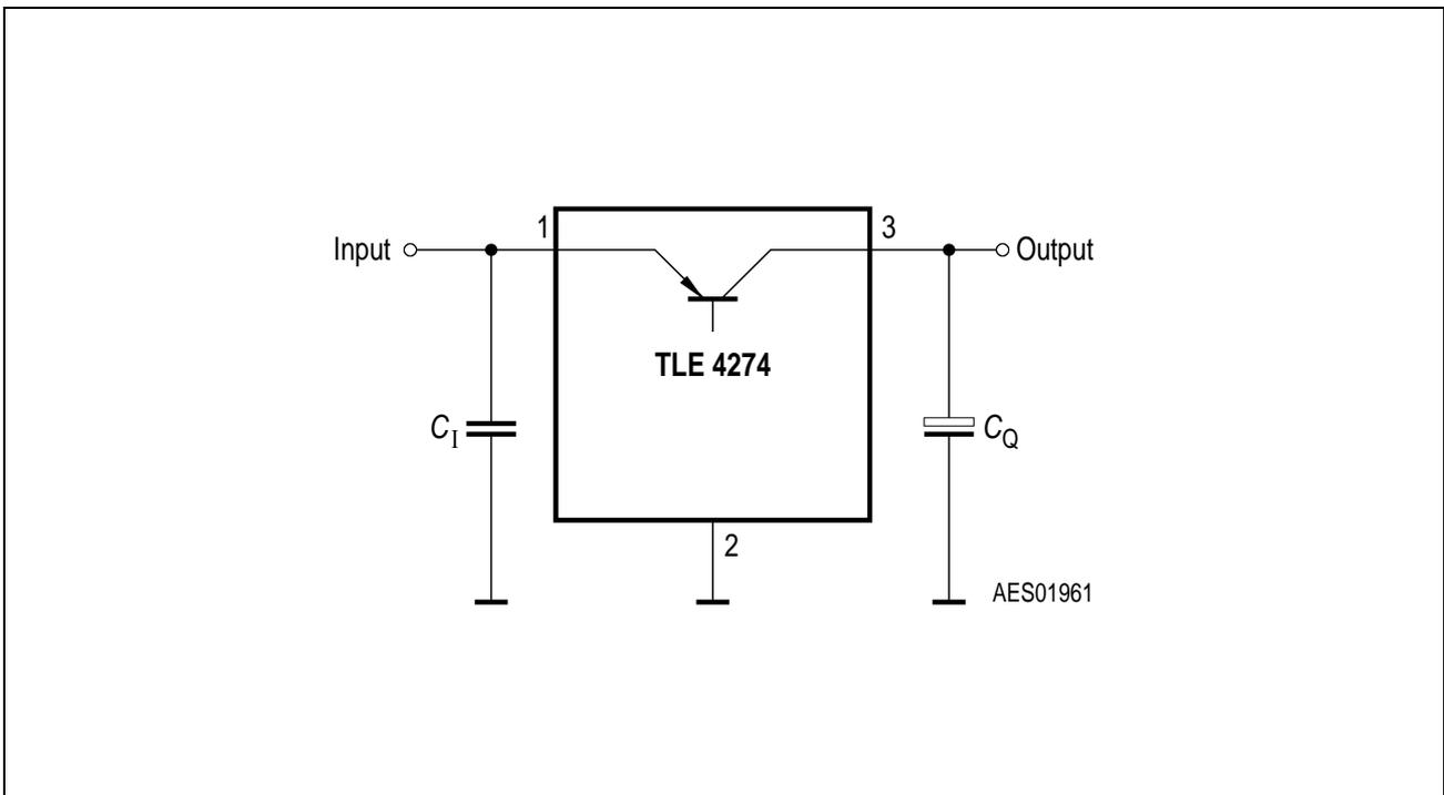
**Figure 4 Application Circuit**
