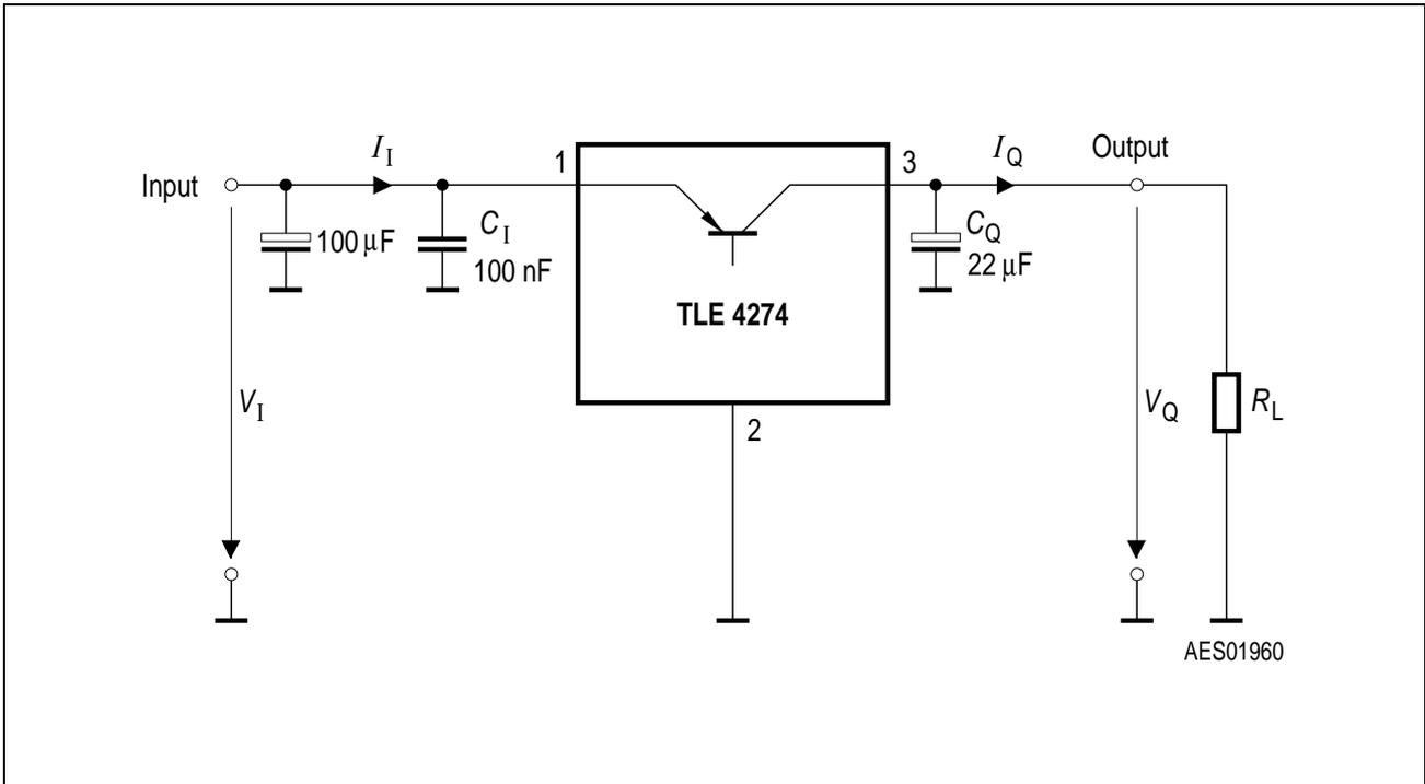
**Figure 3 Measuring Circuit**
