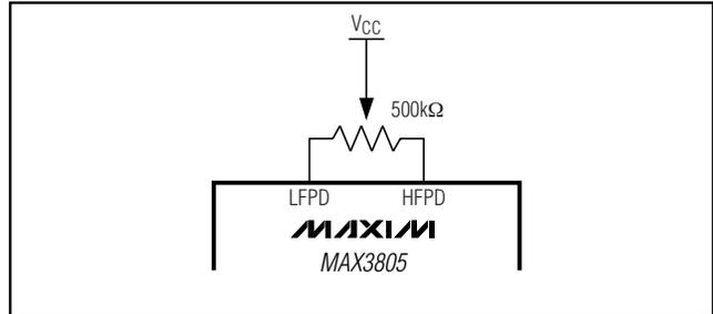
Figure 3. Connecting a Potentiometer Across HFPD and LFPD
