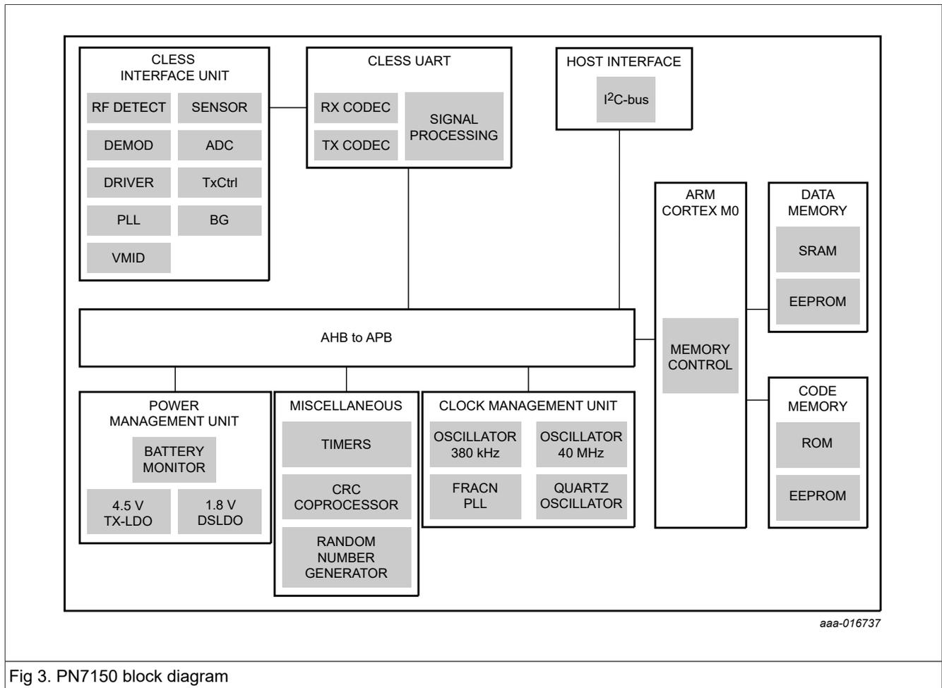
Fig 3. PN7150 block diagram
