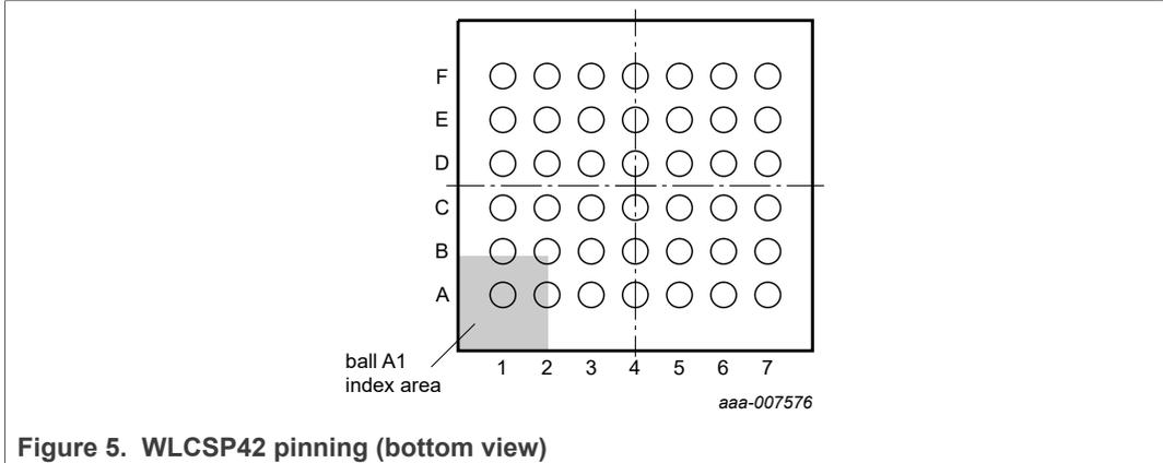
Figure 5. WLCSP42 pinning (bottom view)
