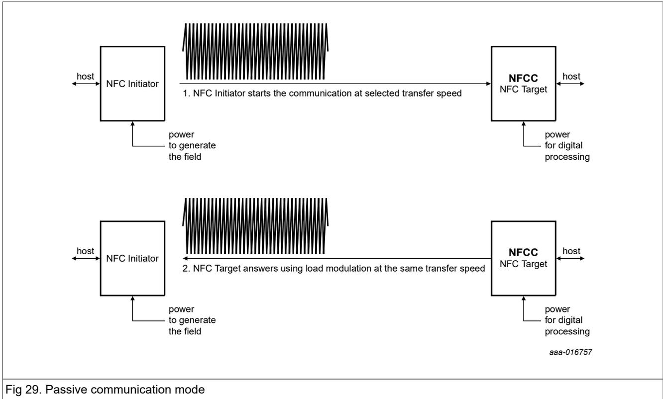
Fig 29. Passive communication mode
