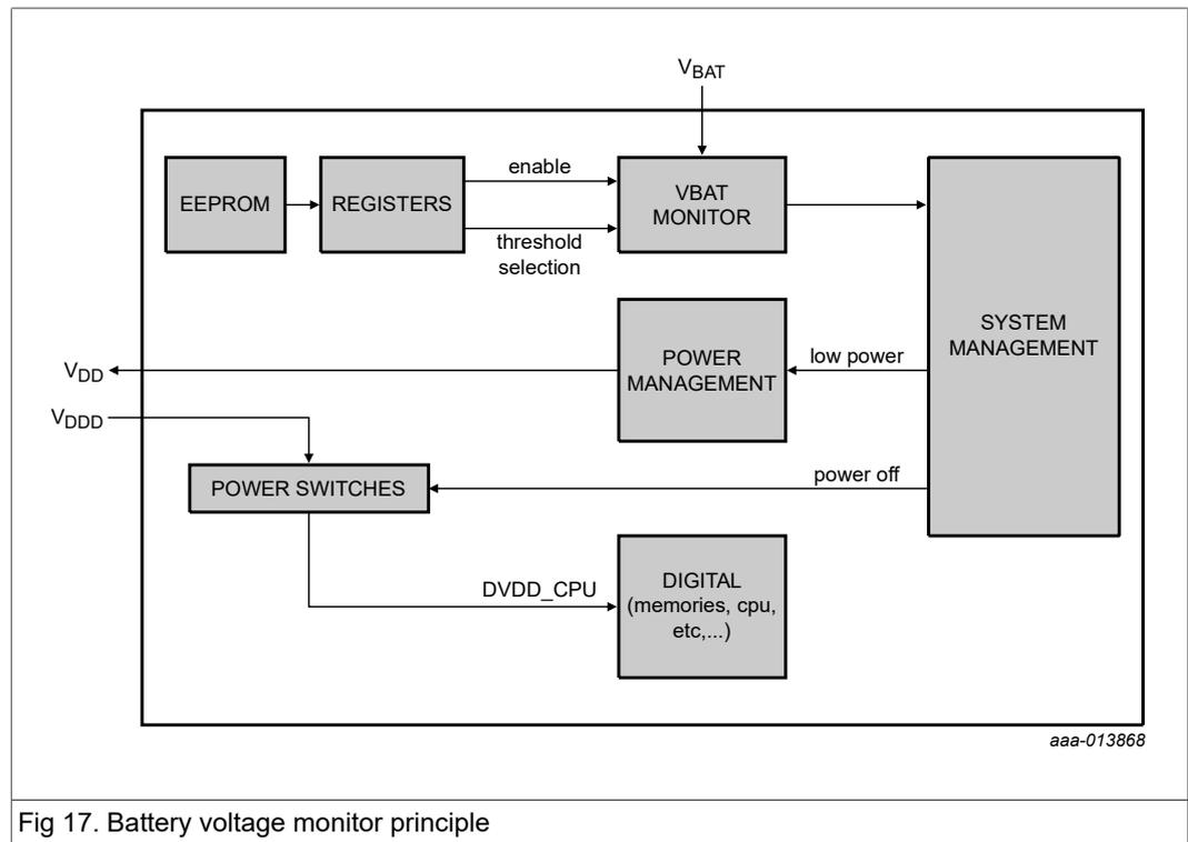
Fig 17. Battery voltage monitor principle
