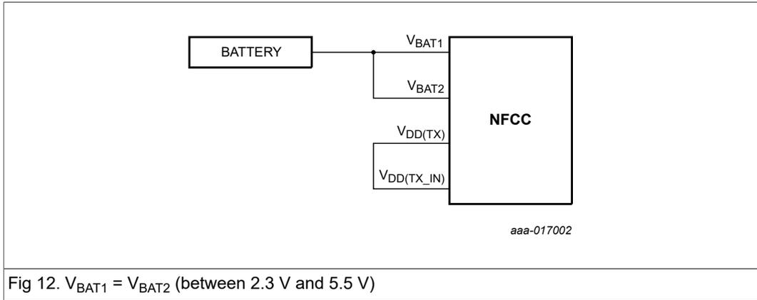
Fig 12.  $V_{BAT1} = V_{BAT2}$  (between 2.3 V and 5.5 V)
