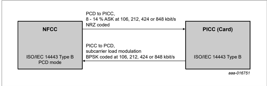
Fig 25. ISO/IEC 14443B Reader/Writer communication mode diagram
