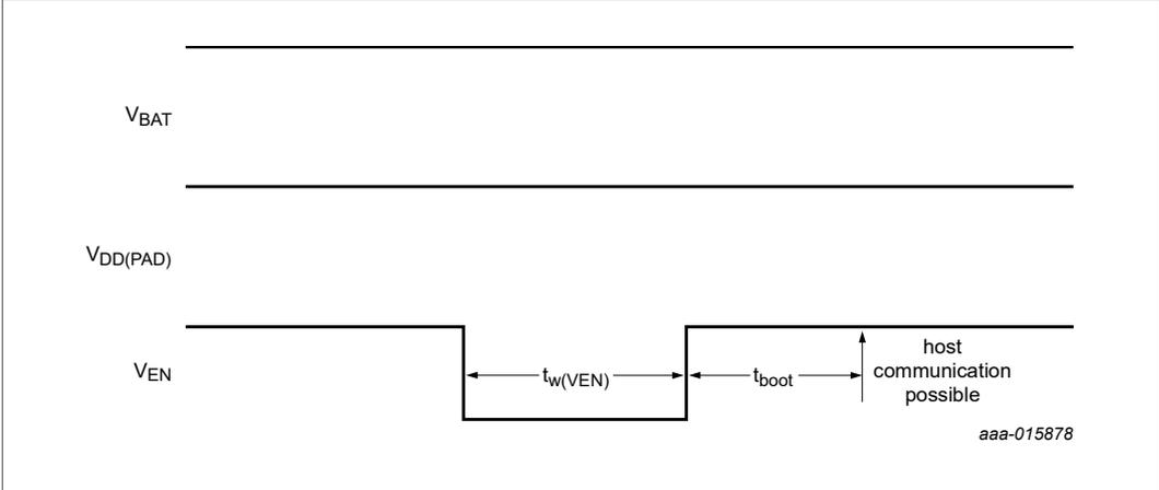
Fig 18. Resetting PN7150 via VEN pin
