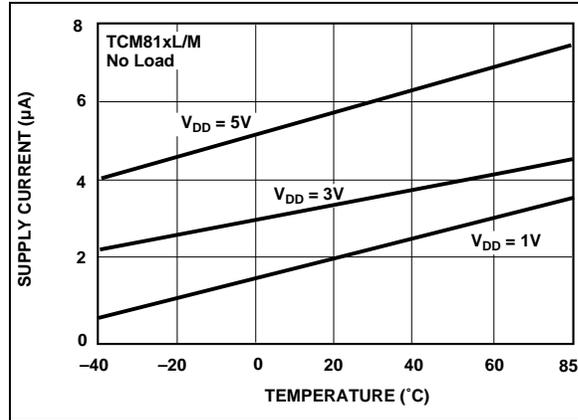
FIGURE 2-4: Supply Current vs. Temperature.
