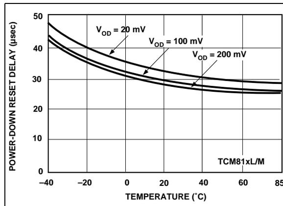
FIGURE 2-5: Power-Down Reset Delay vs. Temperature.
