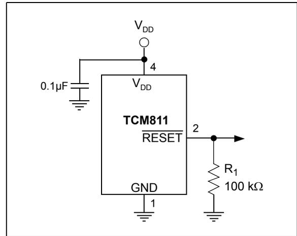
**FIGURE 4-2:** The addition of  $R_1$  at the  $\overline{\text{RESET}}$  output of the TCM811 ensures that the  $\overline{\text{RESET}}$  output is valid to  $V_{DD} = 0\text{V}$ .
