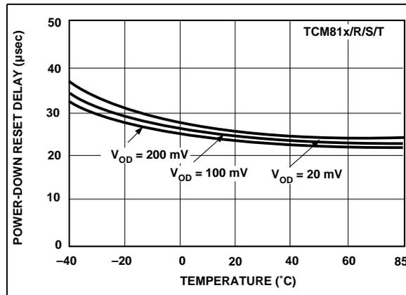
FIGURE 2-6: Power-Down Reset Delay vs. Temperature.
