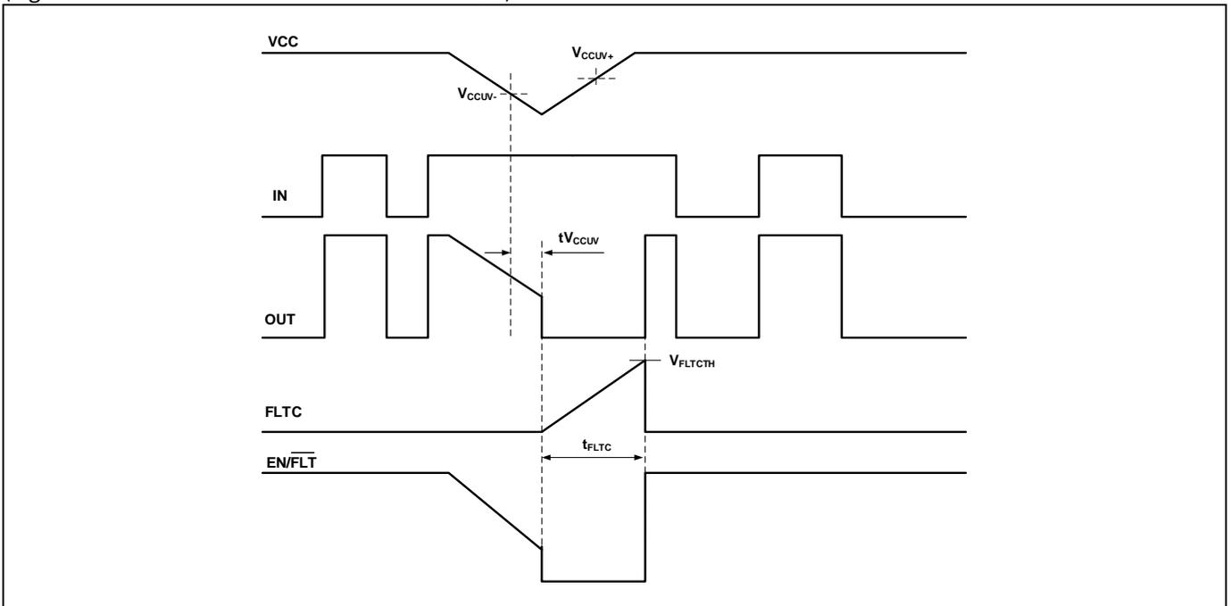
Figure 8 Vcc under voltage protection waveform definitions one
