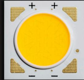
The V Series™ LED Array products deliver high quality light in a compact and cost-effective solid-state lighting package. These chip on board (CoB) arrays can be efficiently driven up to three times the nominal drive current, enabling design flexibility not previously possible. These high flux density light sources are designed to support a wide range of high quality, low cost directional luminaires and replacement lamps for both interior and exterior commercial and residential applications.
