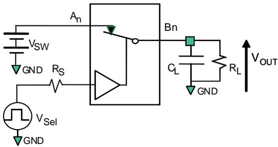
$R_L$ ,  $R_S$ , and  $C_L$  are functions of the application environment (see AC tables for specific values).  $C_L$  includes test fixture and stray capacitance.
