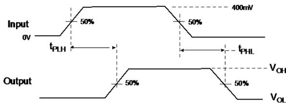
Figure 6. Propagation Delay ( $t_{rly} t_o = 500ps$ )
