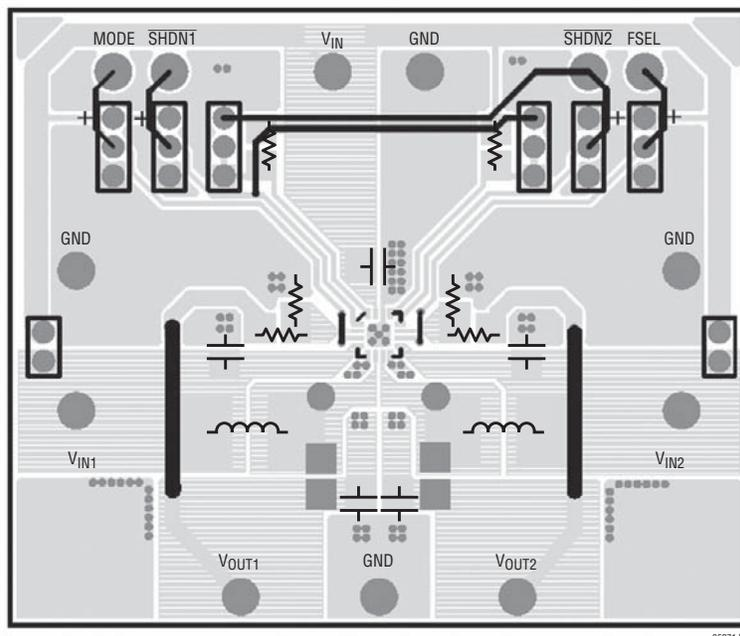
Figure 1. Recommended Component Placement for a Dual-Layer Board
