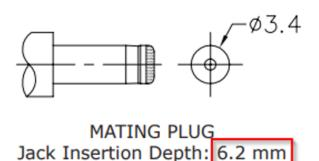
MATING PLUG Jack Insertion Depth: 6.4 mm
