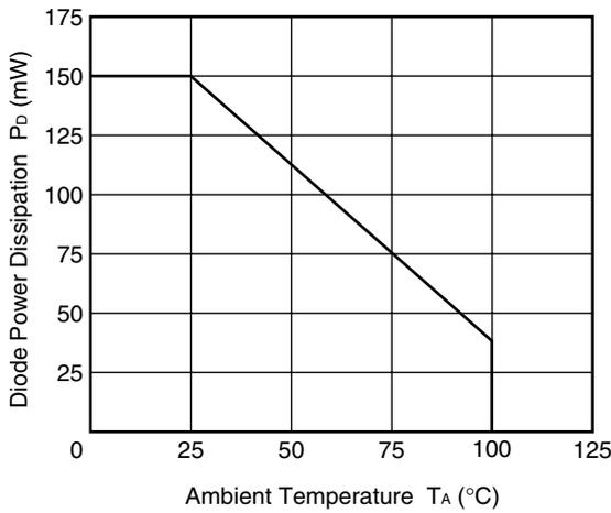
**TRANSISTOR POWER DISSIPATION vs. AMBIENT TEMPERATURE**
