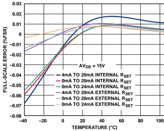
Figure 16. Full-Scale Error vs. Temperature
