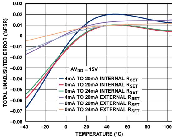
Figure 15. Total Unadjusted Error vs. Temperature
