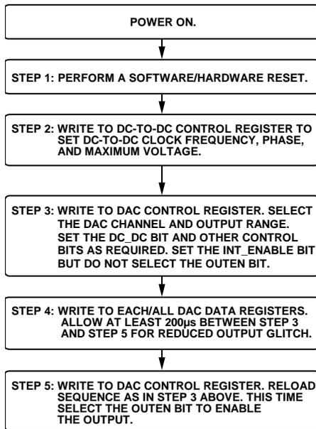
Figure 52. Programming Sequence for Enabling the Output Correctly
