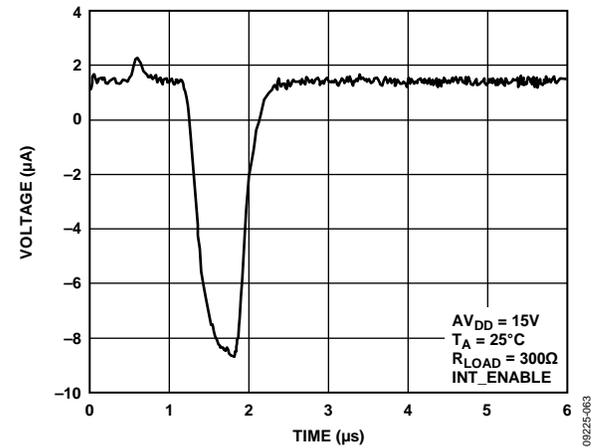
Figure 26. Output Current vs. Time on Output Enable
