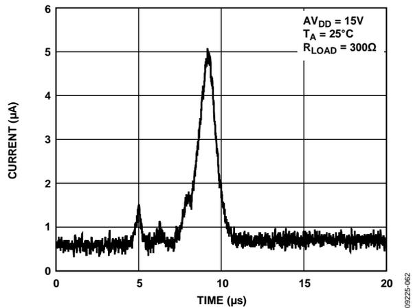
Figure 25. Output Current vs. Time on Power-Up
