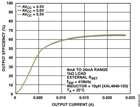
Figure 36. Output Efficiency vs. Output Current (See Figure 57)
