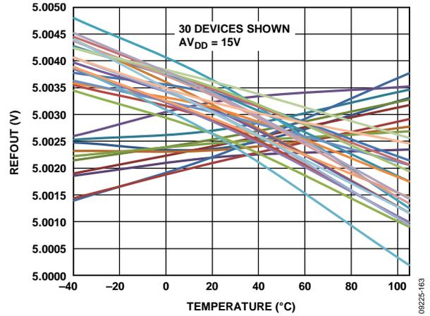
Figure 42. REFOUT vs. Temperature (When the AD5757 is soldered onto a PCB, the reference shifts due to thermal shock on the package. The average output voltage shift is  $-4$  mV. Measurement of these parts after seven days shows that the outputs typically shift back 2 mV toward their initial values. This second shift is due to the relaxation of stress incurred during soldering.)
