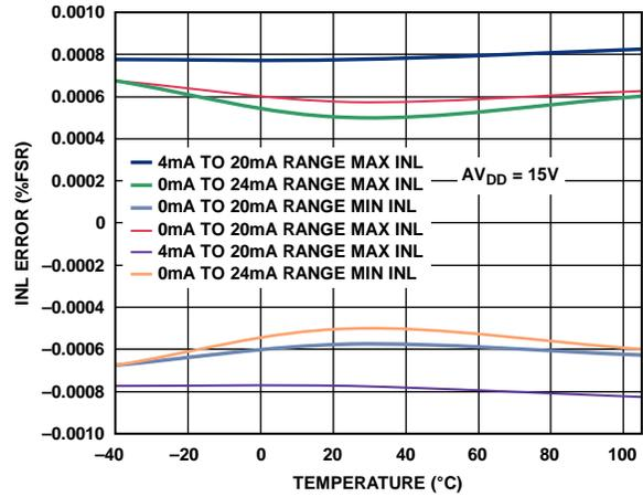
Figure 12. Integral Nonlinearity vs. Temperature, Internal RSET
