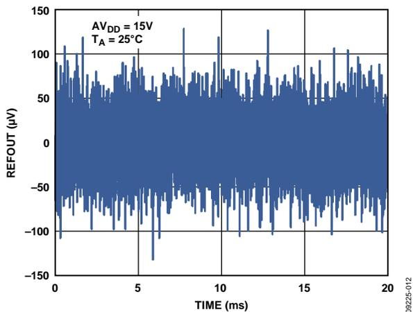
Figure 41. REFOUT Output Noise (100 kHz Bandwidth)
