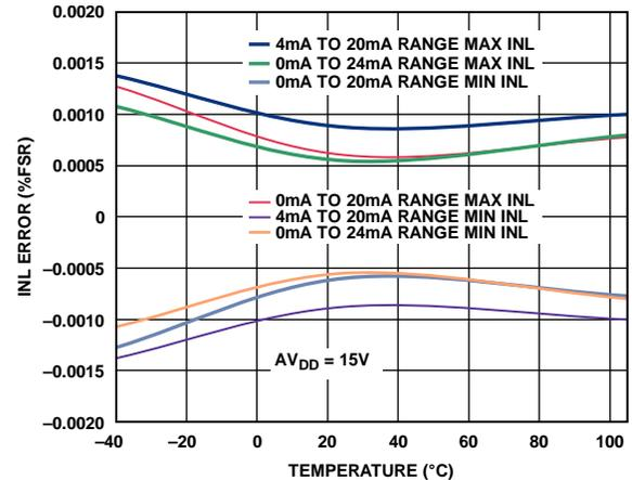
Figure 13. Integral Nonlinearity vs. Temperature, External RSET
