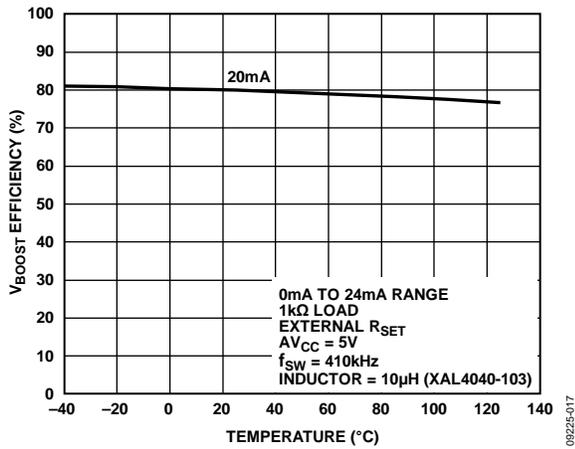
Figure 35. Efficiency at  $V_{BOOST\_x}$  vs. Temperature (See Figure 57)
