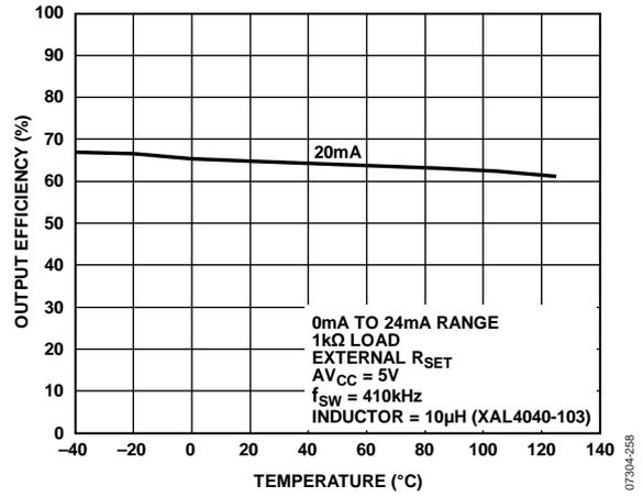
Figure 37. Output Efficiency vs. Temperature (See Figure 57)
