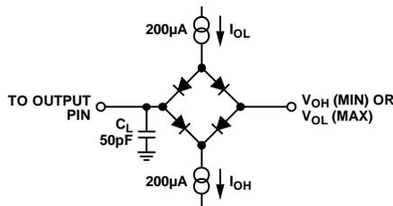
Figure 7. Load Circuit for SDO Timing Diagram
