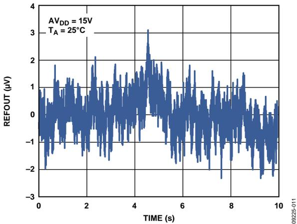
Figure 40. REFOUT Output Noise (0.1 Hz to 10 Hz Bandwidth)
