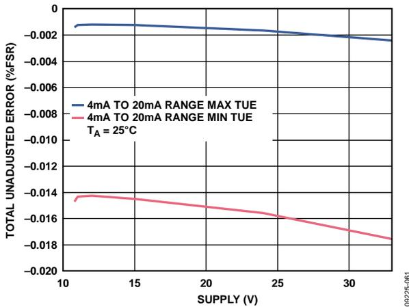
Figure 23. Total Unadjusted Error vs.  $AV_{DD}$ , Internal  $R_{SET}$
