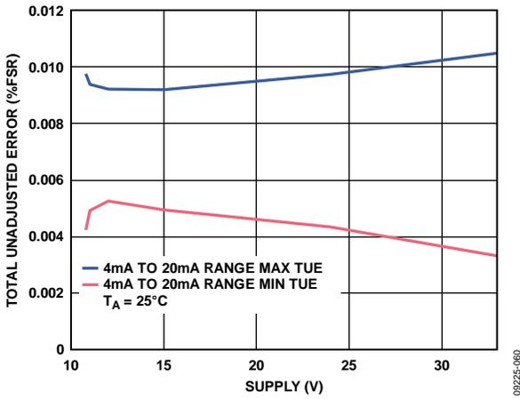
Figure 22. Total Unadjusted Error vs.  $AV_{DD}$ , External  $R_{SET}$
