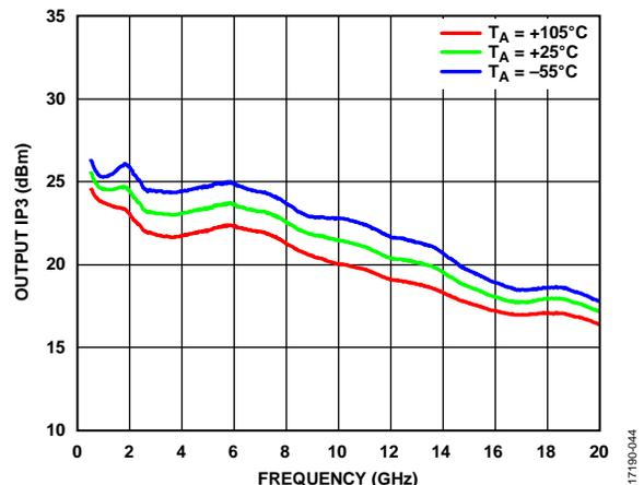
Figure 16. Output IP3 vs. Frequency at Various Temperatures
