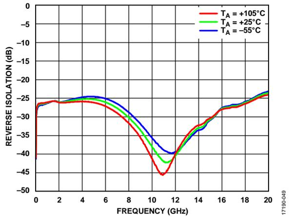
Figure 19. Reverse Isolation vs. Frequency at Various Temperatures
