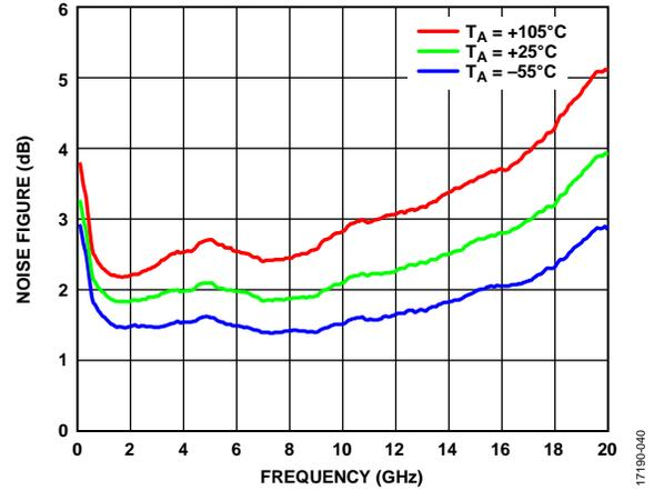
Figure 14. Noise Figure vs. Frequency at Various Temperatures
