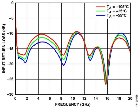
Figure 12. Input Return Loss vs. Frequency at Various Temperatures
