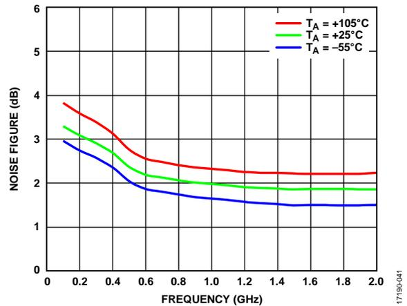
Figure 15. Noise Figure vs. Frequency at Various Temperatures, Low Frequency
