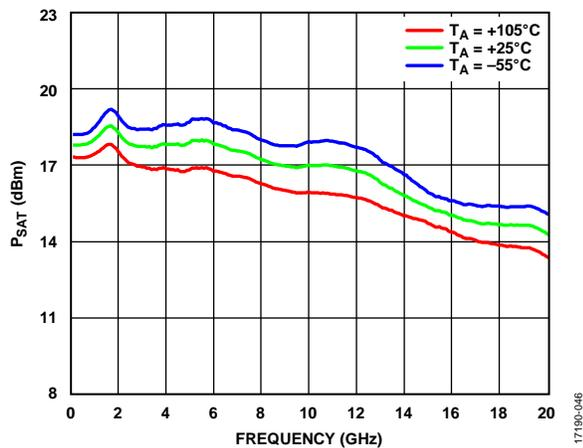
Figure 18. Psat vs. Frequency at Various Temperatures
