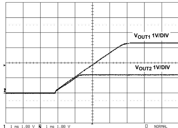
FIGURE 14. PWM1 AND PWM2 OUTPUT TRACKING DURING STARTUP
