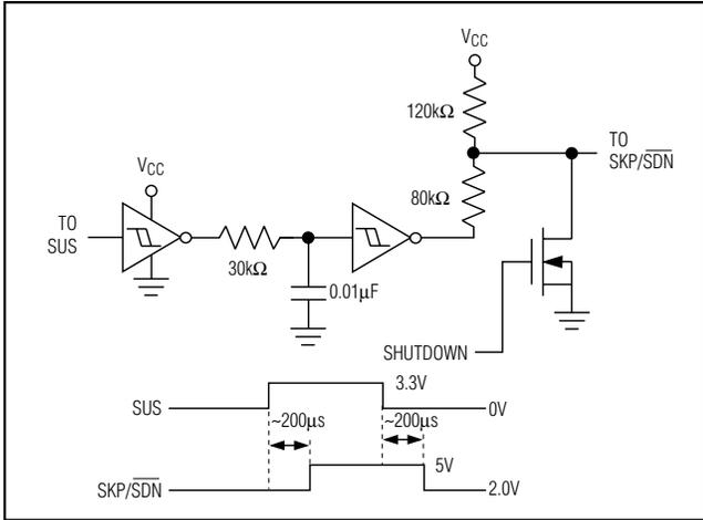
Figure 17. Using Skip Mode During Suspend ( $SKP/SDN = V_{CC}$ )
