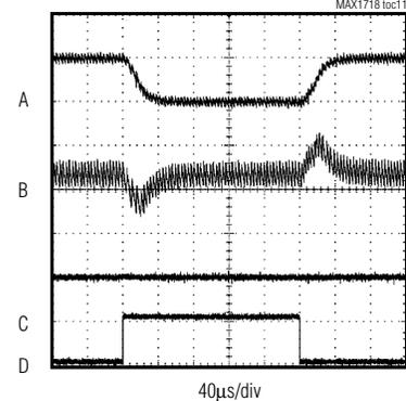
$V_{OUT} = 1.15V$  TO  $1.25V$
