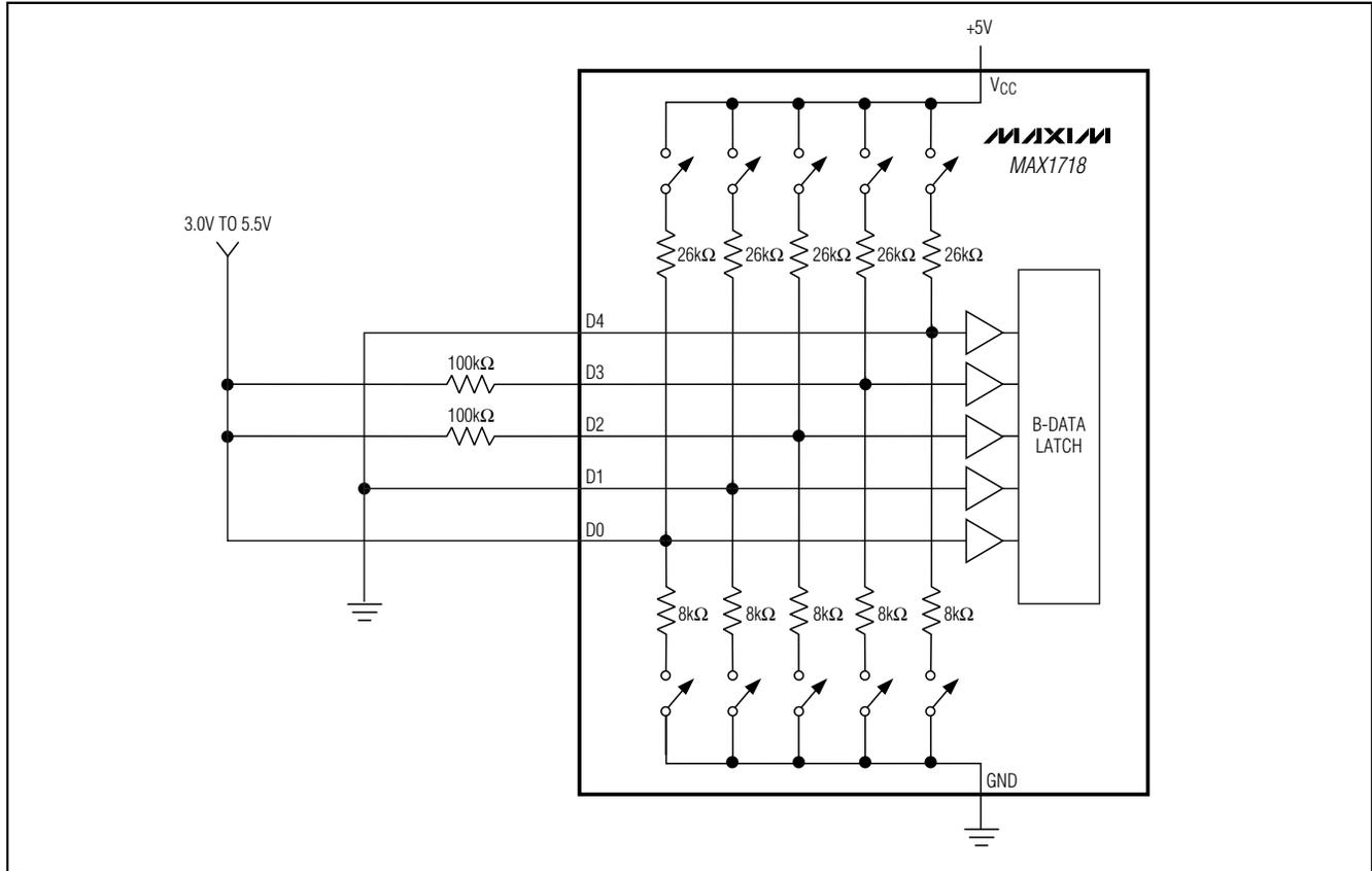
Figure 10. Internal Mux Impedance-Mode Data Test and Latch
