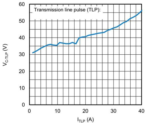
Fig. 7 - Typical Clamping Voltage vs. Peak Pulse Current
