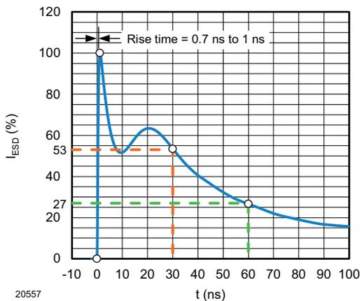
Fig. 1 - ESD Discharge Current Wave Form
