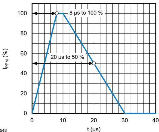
Fig. 2 - 8/20  $\mu\text{s}$  Peak Pulse Current Wave Form
