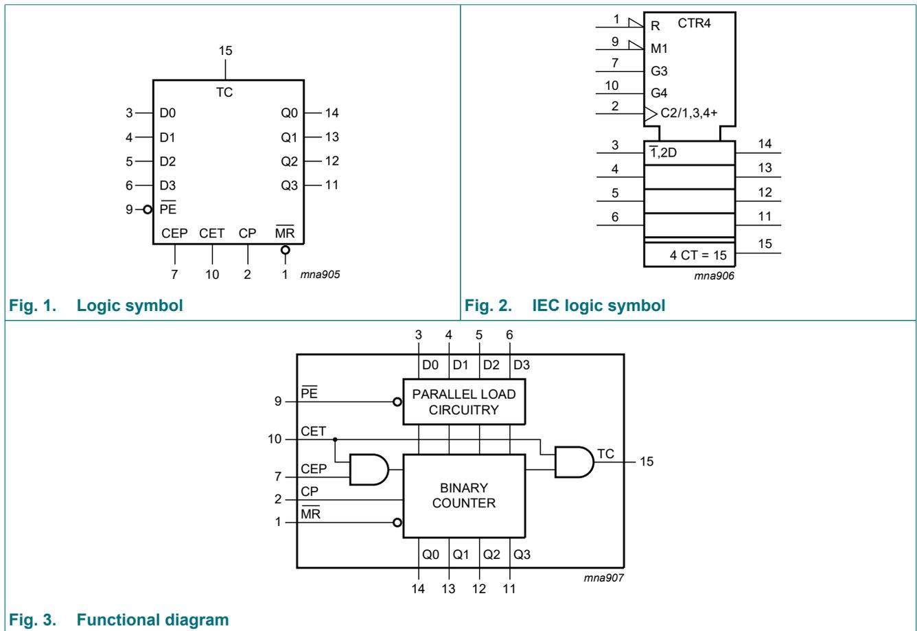
Presetable synchronous 4-bit binary counter; asynchronous reset
