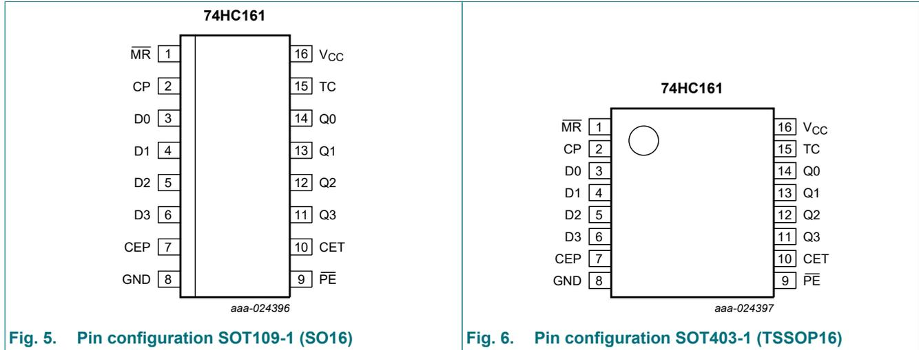
Fig. 5. Pin configuration SOT109-1 (SO16)
