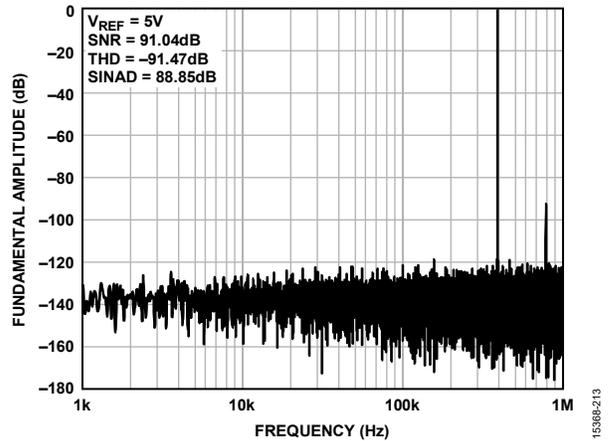
Figure 16. 400 kHz,  $-0.5\text{ dBFS}$  Input Tone FFT
