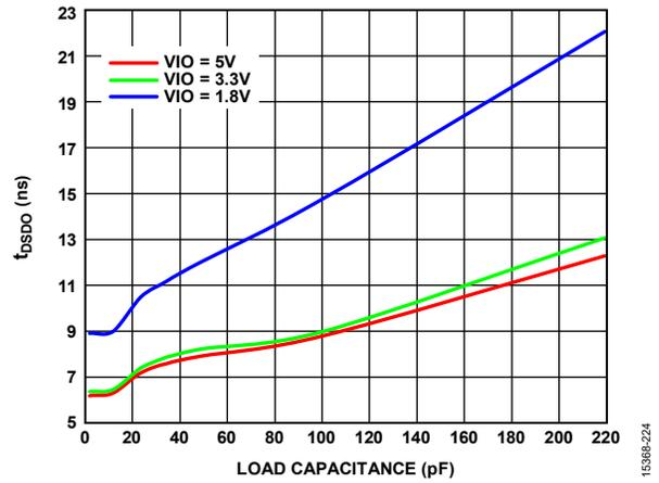
Figure 36. t<sub>DSDO</sub> vs. Load Capacitance
