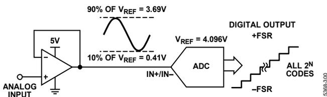
Figure 45. Span Compression
