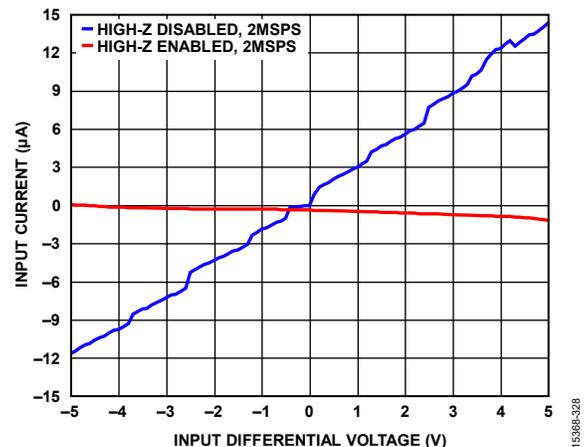
Figure 2. Input Current vs. Input Differential Voltage
