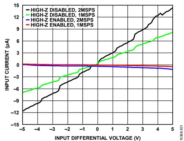
Figure 28. Analog Input Current vs. Input Differential Voltage
