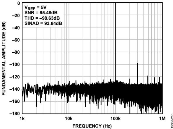
Figure 13. 100 kHz,  $-0.5\text{ dBFS}$  Input Tone FFT
