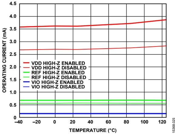
Figure 30. Operating Current vs. Temperature, AD4005, 1 MSPS
