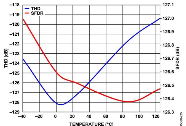
Figure 22. THD and SFDR vs. Temperature,  $f_{IN} = 1$  kHz
