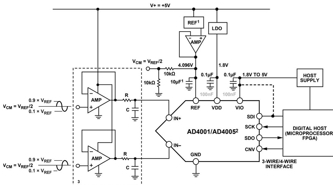
1SEE THE VOLTAGE REFERENCE INPUT SECTION FOR REFERENCE SELECTION.  $C_{REF}$  IS USUALLY A 10μF CERAMIC CAPACITOR (X7R).
