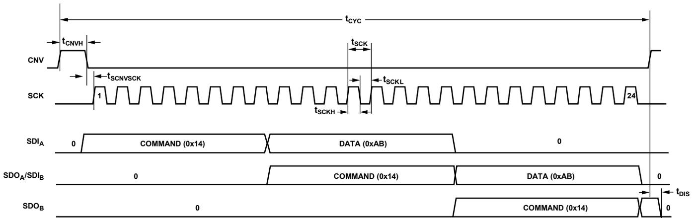
Figure 50. Register Write Timing Diagram, Daisy-Chain Mode
