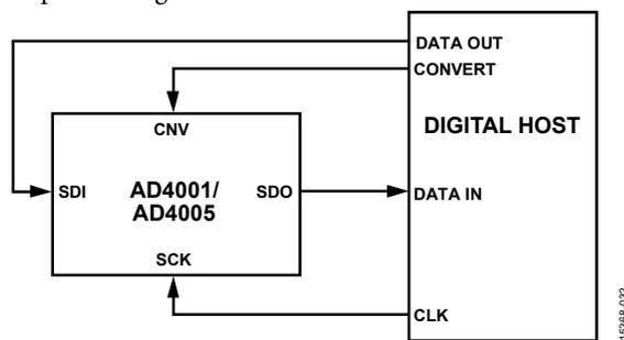
Figure 58. CS Mode, 4-Wire Turbo Mode Connection Diagram
