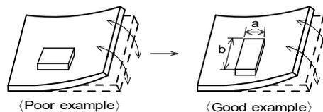
(2) Components location on PCB separation
