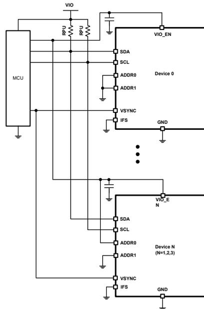
**Figure 8-16. I<sup>2</sup>C Multiple Devices Connection**
