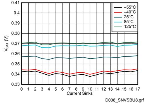
**Figure 7-4.  $V_{SAT}$  vs Current Sinks (50 mA)**
