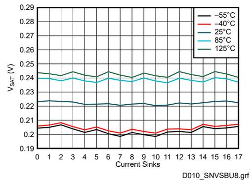
**Figure 7-6.  $V_{SAT}$  vs Current Sinks (10 mA)**
