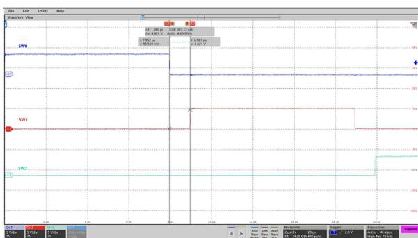
Switch blank time  $t_{SW\_BLK} = 1 \mu s$
