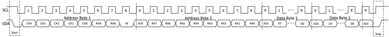
**Figure 8-14. I<sup>2</sup>C Write Timing**
