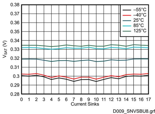
**Figure 7-5.  $V_{SAT}$  vs Current Sinks (30 mA)**
