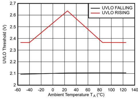
**Figure 7-1.  $V_{CC}$  UVLO Rising and Falling Thresholds**
