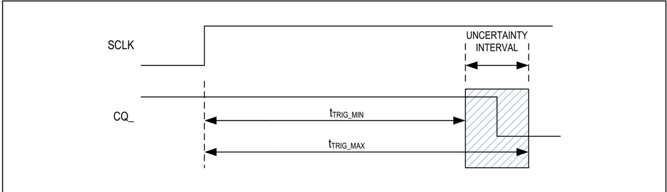
Figure 13. Trigger Delay
