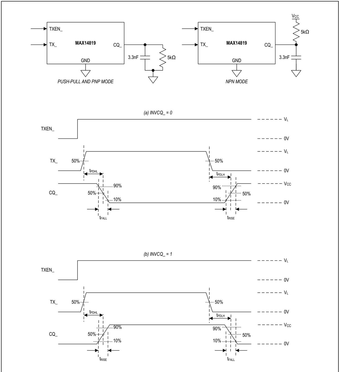
Figure 1. C/Q Driver Propagation Delays and Rise/Fall Times
