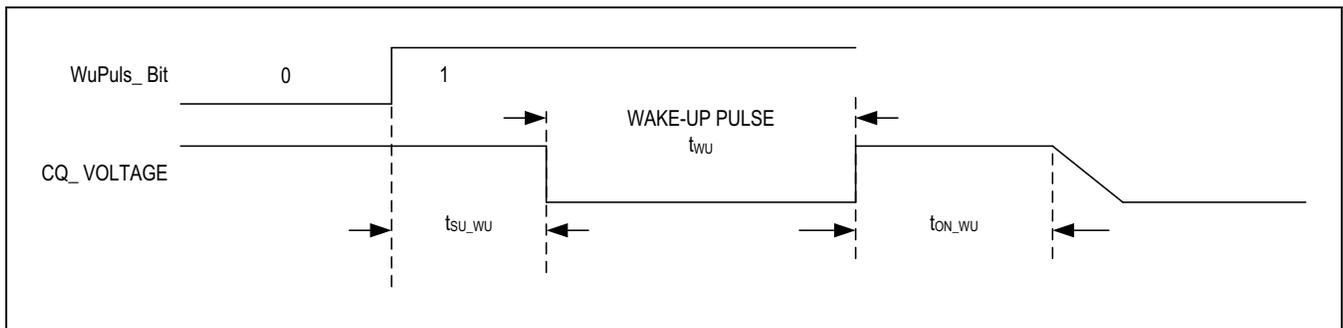
Figure 9. Wake-Up Timing
