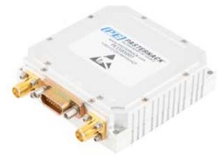
VHF/UHF BiDirectional Amplifier, 225 MHz to 512 MHz 16W Psat, 35% Efficiency, 8 usec Switching, 36dB Tx Gain, Manual T/R Control, SMA
