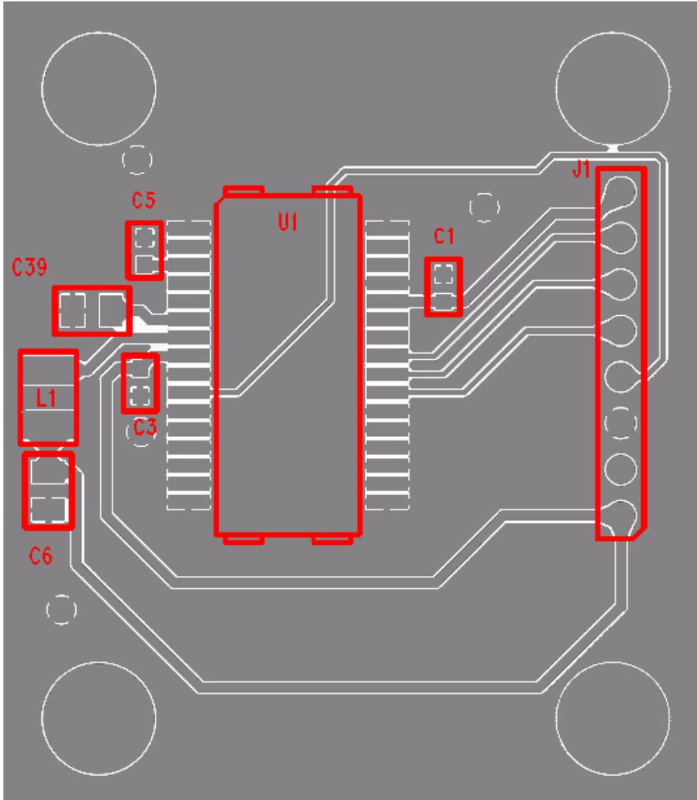
Figure 11. Example layout for SCR1100.
