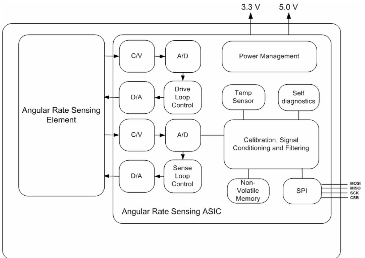
Figure 1. SCR1100 component block diagram.
