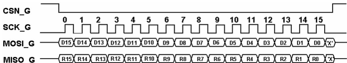
Figure 4. SCR1100 angular rate sensor 16-bit data transmission.
