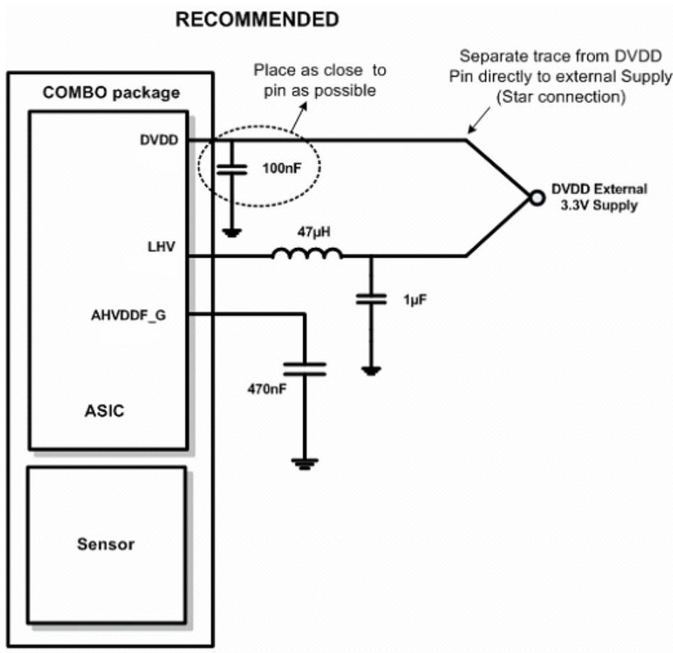
Figure 10. Layout recommendations for DVDD\_G/LHV pin decoupling.
