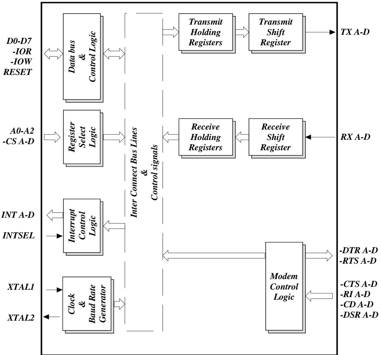
Figure 3, Block Diagram in 68 Mode
