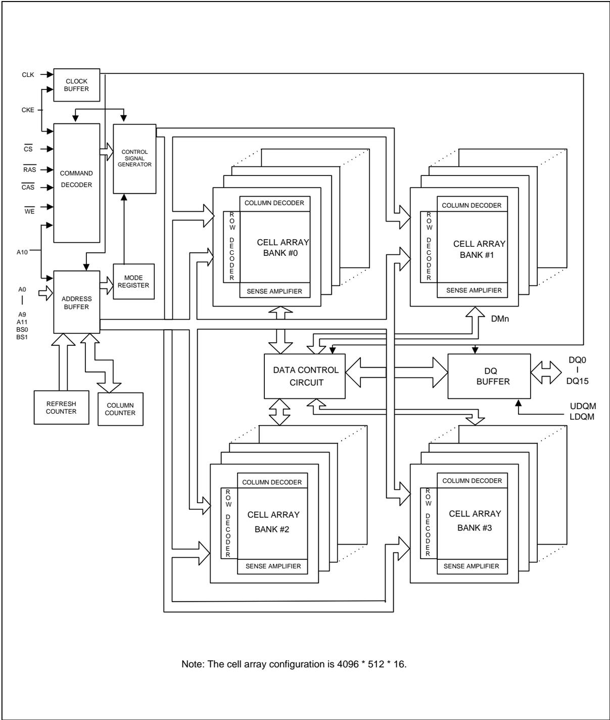
Note: The cell array configuration is 4096 \* 512 \* 16.
