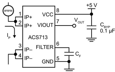
Application 1. The ACS713 outputs an analog signal,  $V_{OUT}$ , that varies linearly with the unidirectional DC primary sampled current,  $I_P$ , within the range specified.  $C_F$  is recommended for noise management, with values that depend on the application.
