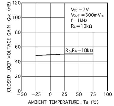
Fig.7 Closed loop voltage gain vs. ambient temperature
