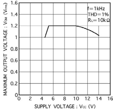
Fig.12 Maximum output voltage vs. power supply voltage
