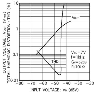
Fig.11 Input/output characteristics
