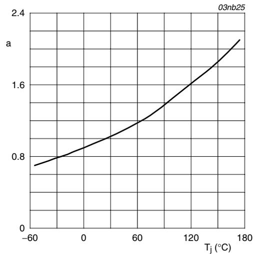
$$a = \frac{R_{DSon}}{R_{DSon(25^\circ\text{C})}}$$
