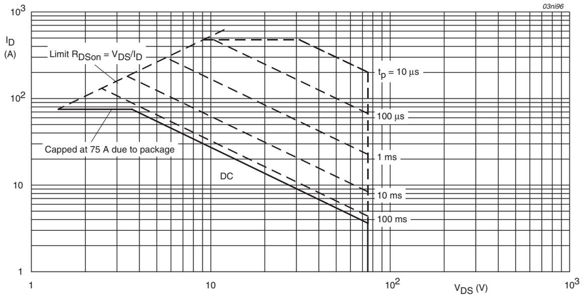
$T_{mb} = 25^\circ C; I_{DM}$  is single pulse
