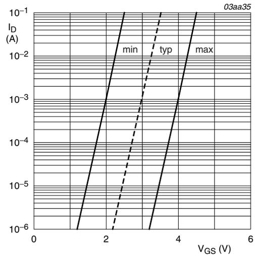
$T_j = 25\text{ °C}; V_{DS} = 5\text{ V}$
