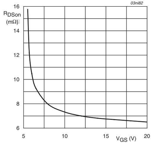
$T_j = 25^\circ\text{C}; I_D = 50\text{A}$
