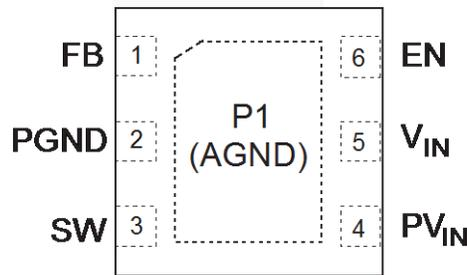
Figure 2. Pin Assignments
