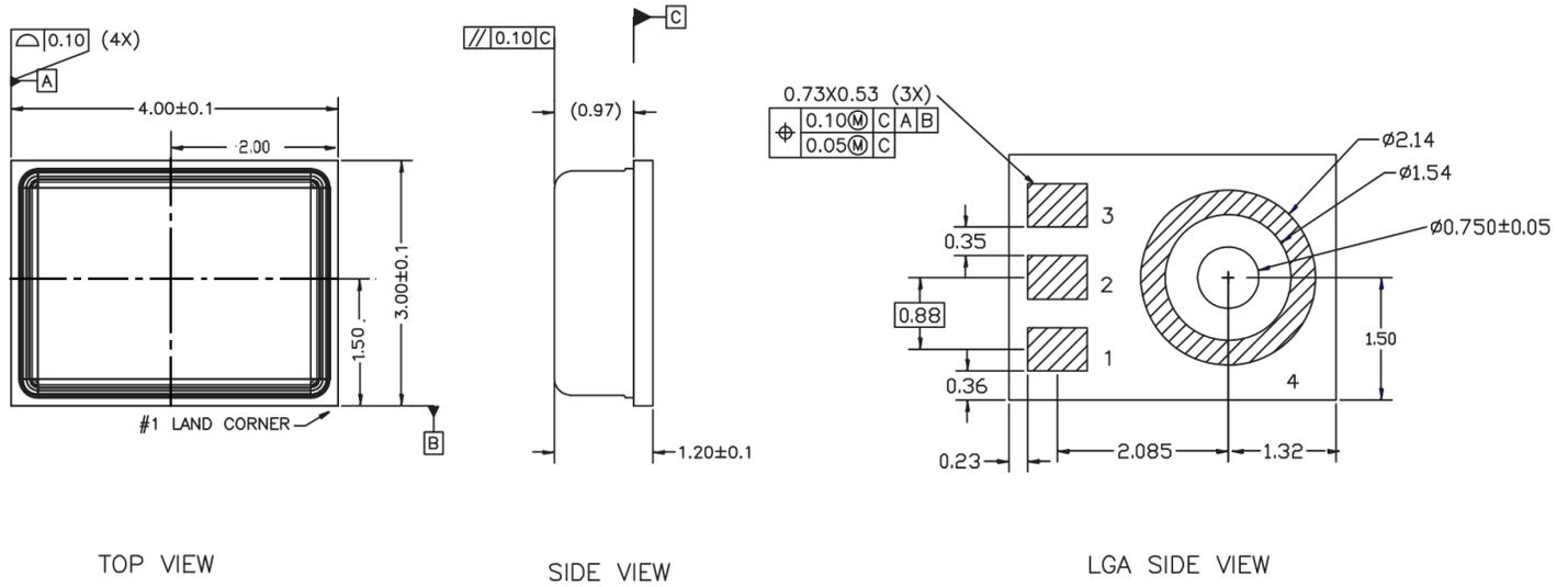
**Figure 11. 4-Terminal Chip Array Small Outline No Lead Cavity**
