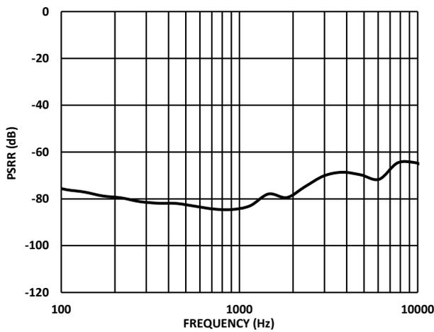
**Figure 5. Power-Supply Rejection Ratio (PSRR) vs. Frequency**
