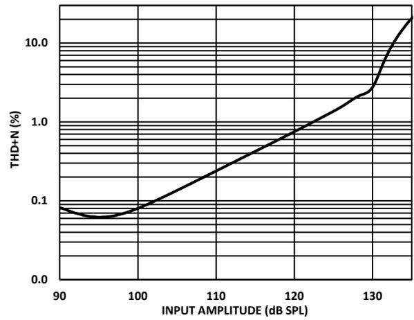
**Figure 4. THD + N vs. Input Level**
