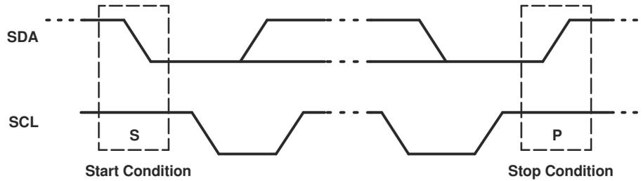
**Figure 9-3. Definition Of Start And Stop Conditions**
