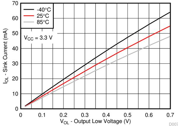
Figure 7-7. I/O Sink Current vs Output Low Voltage for Different Temperature (T<sub>A</sub>) for V<sub>CC</sub> = 3.3 V
