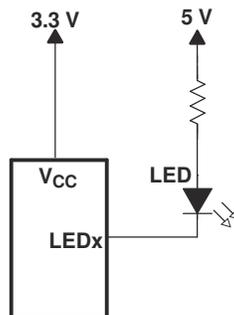
Figure 10-3. Device Supplied By A Lower Voltage
