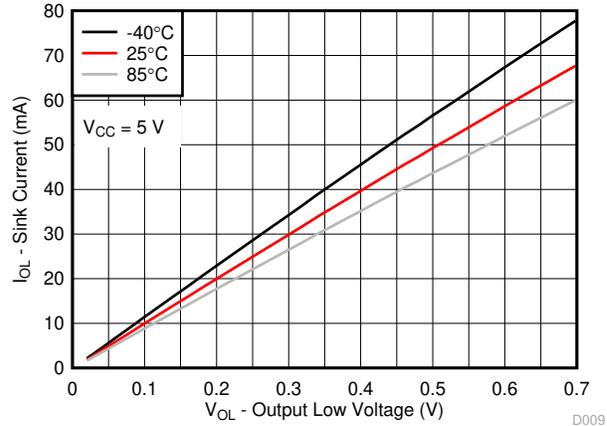
Figure 7-8. I/O Sink Current vs Output Low Voltage for Different Temperature (T<sub>A</sub>) for V<sub>CC</sub> = 5 V
