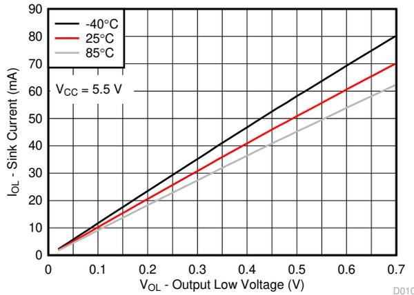
Figure 7-9. I/O Sink Current vs Output Low Voltage for Different Temperature (T<sub>A</sub>) for V<sub>CC</sub> = 5.5 V
