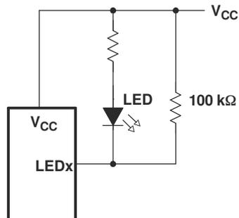
Figure 10-2. High-Value Resistor In Parallel With The Led
