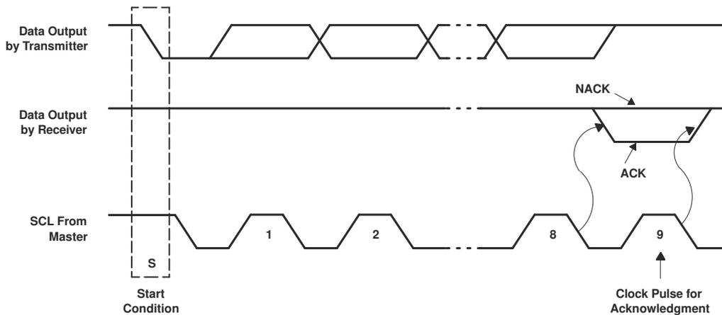
**Figure 9-5. Acknowledgment On I<sup>2</sup>C Bus**
