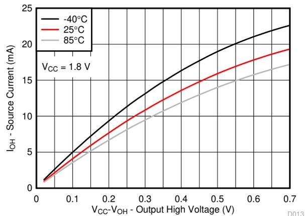
Figure 7-12. I/O Source Current vs Output High Voltage for Different Temperature (T<sub>A</sub>) for V<sub>CC</sub> = 1.8 V
