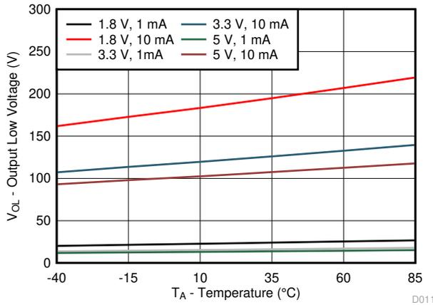
Figure 7-10. I/O Low Voltage vs Temperature for Different V<sub>CC</sub> and I<sub>OL</sub>
