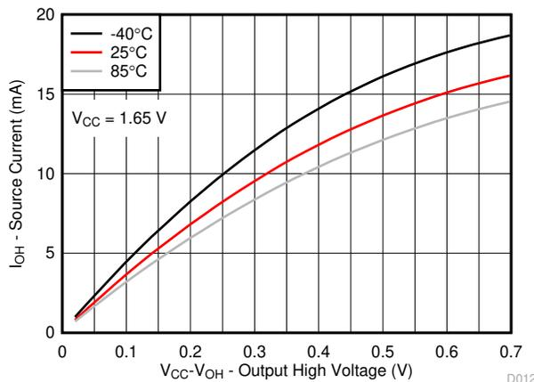
Figure 7-11. I/O Source Current vs Output High Voltage for Different Temperature (T<sub>A</sub>) for V<sub>CC</sub> = 1.65 V
