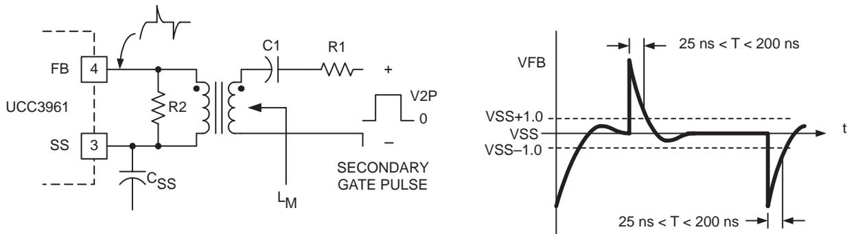
**Figure 3. Pulse Edge Transmission Circuit**
