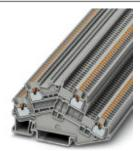
Double-level terminal block, Cross section: 0.14 mm² - 1.5 mm², AWG: 26 - 14, Connection type: Push-in connection, Width: 3.5 mm, Color: gray, Mounting type: NS 35/7,5, NS 35/15
