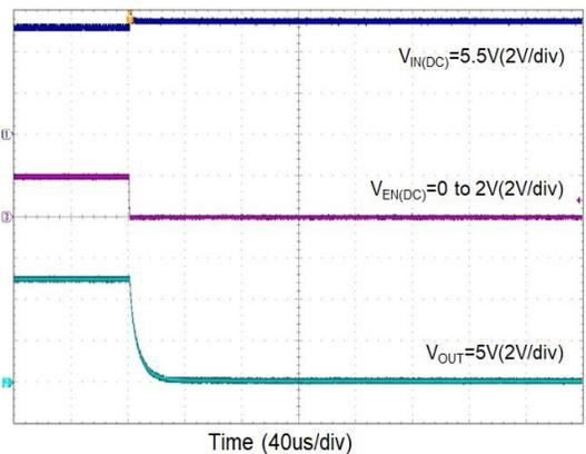
**Typical Characteristics** ( $C_{IN} = C_{OUT} = 1\mu F$ ) (continued)
