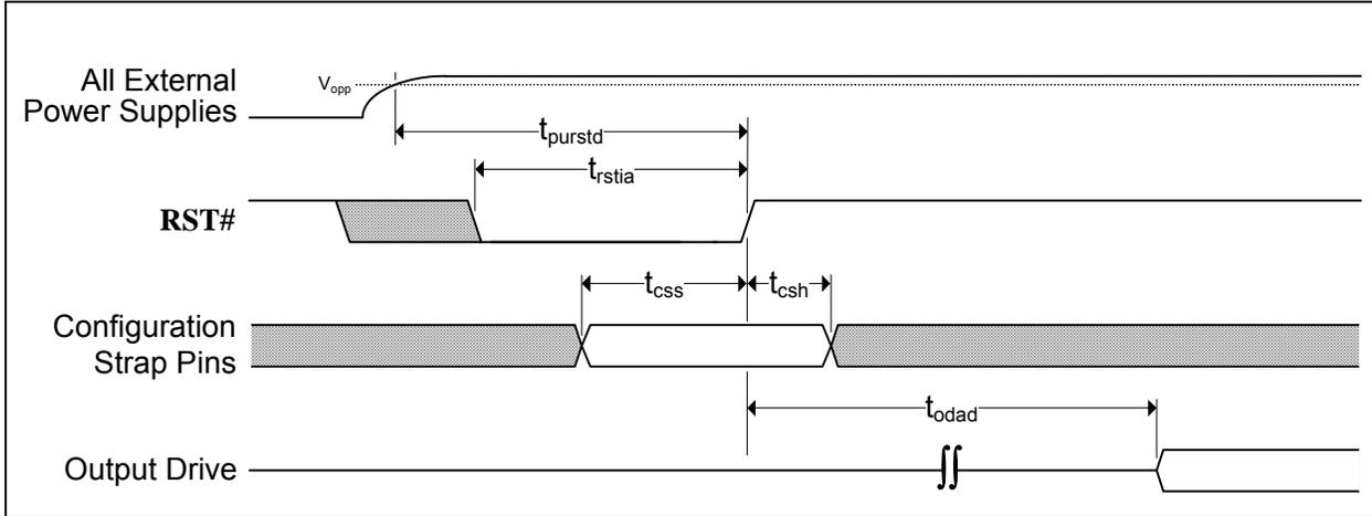
**TABLE 19-11: RST# PIN CONFIGURATION STRAP LATCHING TIMING VALUES**
