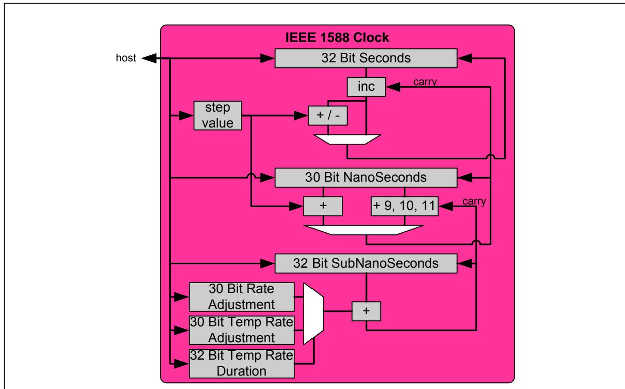
The 1588 Clock consists of a 32-bit wide seconds portion and a 30-bit wide nanoseconds portion. Running at a nominal reference frequency of 100MHz, the nanoseconds portion is normally incremented by a value of 10 every reference clock period. Upon reaching or exceeding its maximum value of  $10^9$ , the nanoseconds portion rolls over to or past zero and the seconds portion is incremented.
