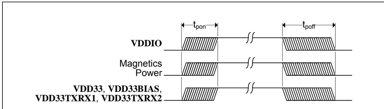
**FIGURE 19-3: POWER SEQUENCE TIMING - EXTERNAL REGULATORS**
