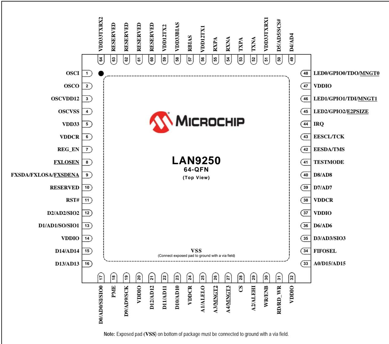
**Note:** When a “#” is used at the end of the signal name, it indicates that the signal is active low. For example, **RST#** indicates that the reset signal is active low.
