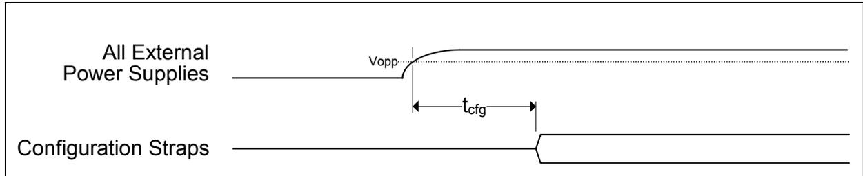
**TABLE 19-12: POWER-ON CONFIGURATION STRAP LATCHING TIMING VALUES**
