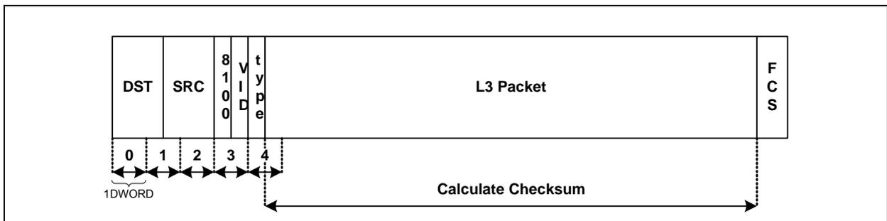
**FIGURE 11-5: ETHERNET FRAME WITH LENGTH FIELD AND SNAP HEADER**
