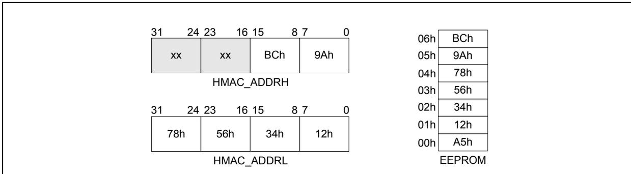
**Note:** By convention, the right nibble of the left most byte of the Ethernet address (in this example, the 2 of the 12h) is the most significant nibble and is transmitted/received first.
