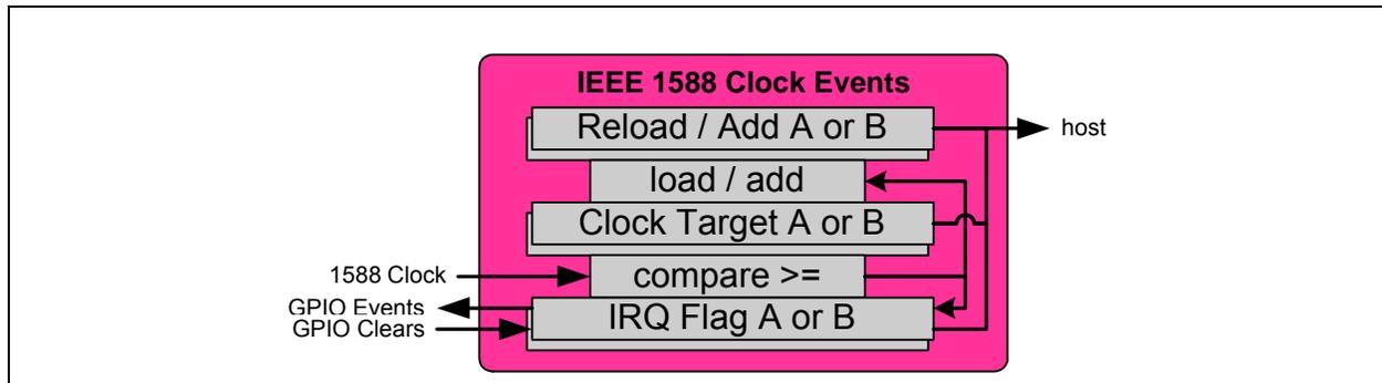
For each clock event channel, a comparator compares the 1588 Clock with a Clock Target loaded in the [1588 Clock Target x Seconds Register \(1588\\_CLOCK\\_TARGET\\_SEC\\_x\)](#) and [1588 Clock Target x NanoSeconds Register \(1588\\_CLOCK\\_TARGET\\_NS\\_x\)](#).
