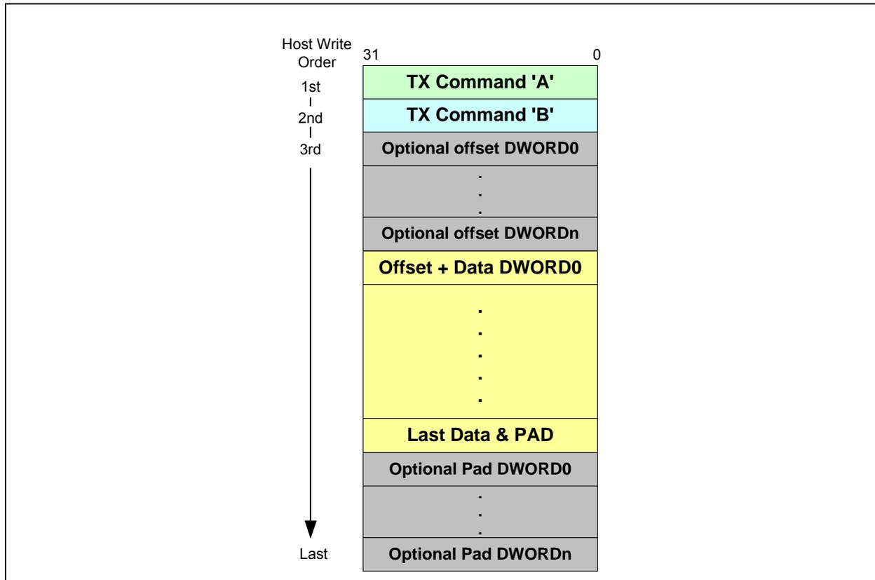
Figure 11-11 shows the TX Buffer as it is written into the device. It should be noted that not all of the data shown in this diagram is actually stored in the TX Data FIFO. This must be taken into account when calculating the actual TX Data FIFO usage. Please refer to Section 11.11.5, "Calculating Actual TX Data FIFO Usage" for a detailed explanation on calculating the actual TX Data FIFO usage.
