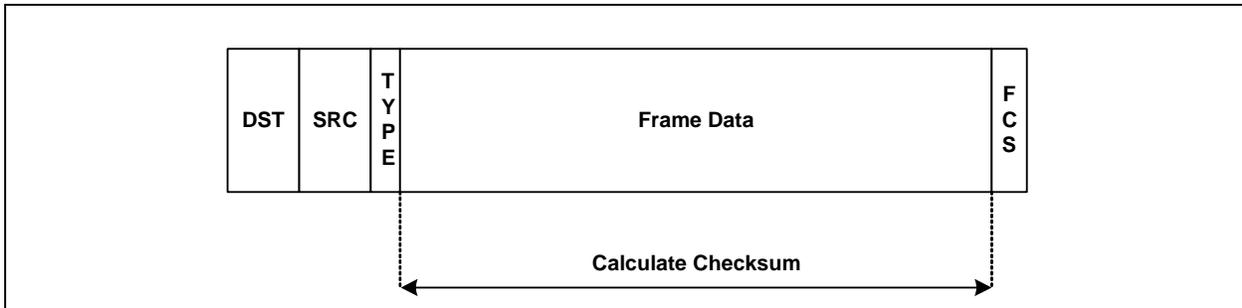
In mode 1, the RXCOE supports VLAN tags and a SNAP header. In this mode, the RXCOE calculates the checksum at the start of L3 packet. The VLAN1 tag register is used by the RXCOE to indicate what protocol type is to be used to indicate the existence of a VLAN tag. This value is typically 8100h.
