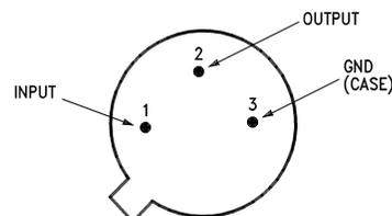
Figure 1. TO Metal Can Package (NDT)
