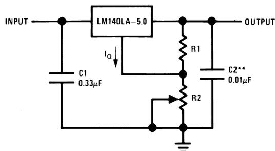
$$V_{\text{OUT}} = 5V + (5V/R1 + I_O) R2$$
