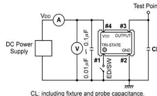
CL: including fixture and probe capacitance.
