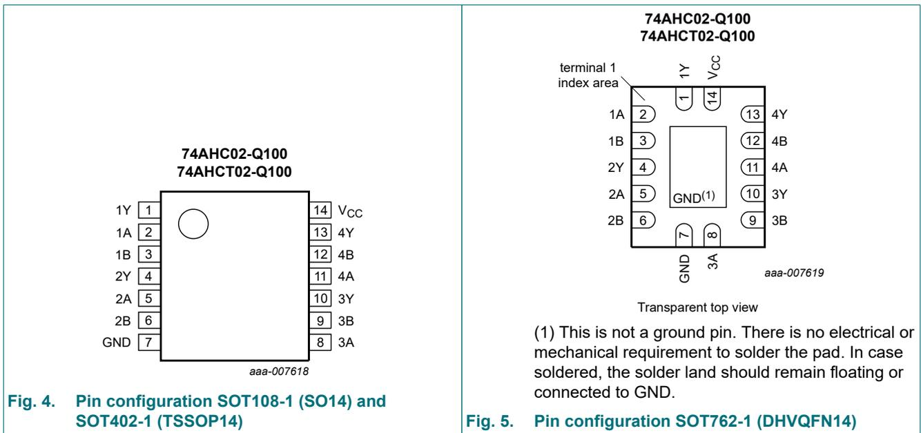
Fig. 4. Pin configuration SOT108-1 (SO14) and SOT402-1 (TSSOP14)
