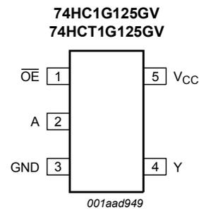
Figure 5. Pin configuration SC-74A
