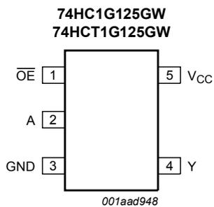
Figure 4. Pin configuration TSSOP5
