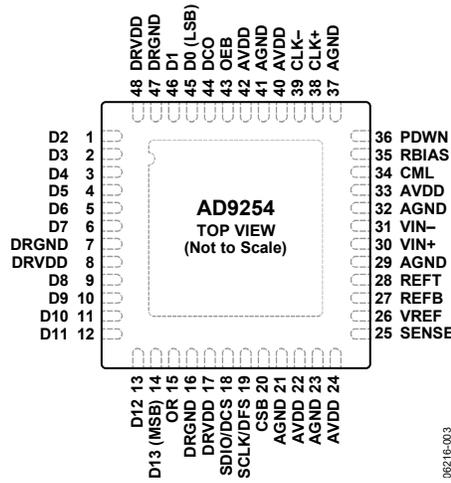
Figure 3. Pin Configuration
