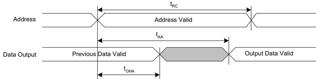
**Figure 5. SRAM Read Cycle #2 ( $\overline{CE}$  and  $\overline{OE}$  Controlled)** [16, 18]
