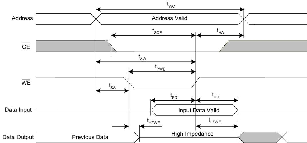
Figure 7. SRAM Write Cycle #2 ( $\overline{CE}$  Controlled) [19, 20, 21]
