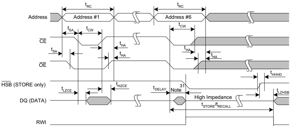
Figure 10. AutoStore Enable / Disable Cycle <sup>[30]</sup>
