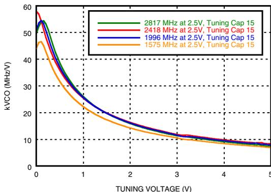
**Figure 6. Typical Tuning Voltage After Calibration at Fo**
