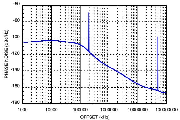
**Figure 15. Fractional-N Exact Frequency Mode ON Performance at 2113.5 MHz<sup>[7]</sup>**
