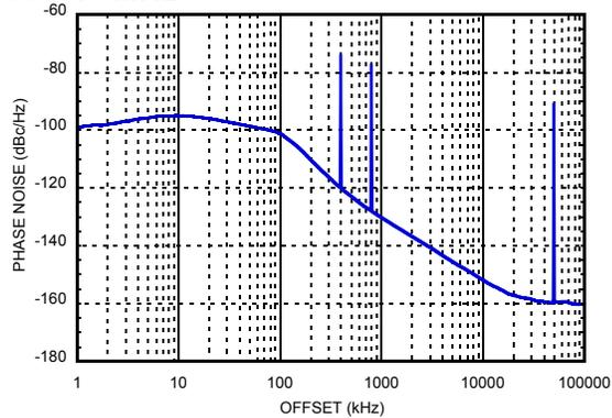
**Figure 14. Integer Boundary Spur at 3900.4 MHz<sup>[5]</sup>**
