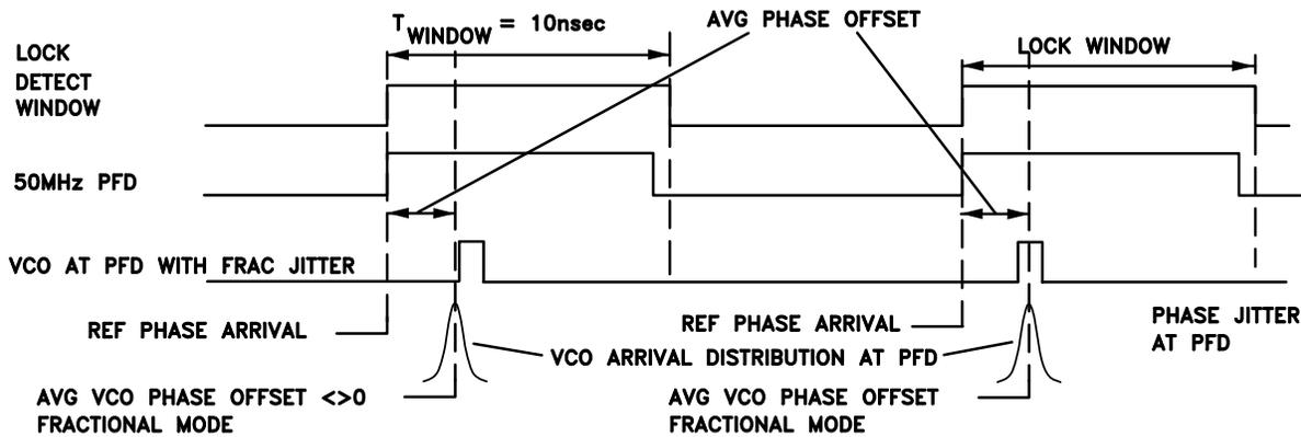
Figure 41. Lock Detect Window - Fractional Mode with Offset
