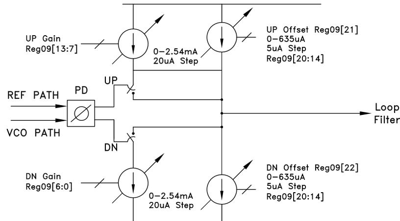
Figure 43. Charge Pump Gain & Offset Control
