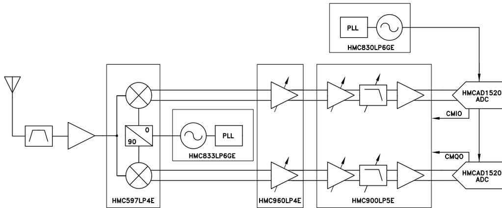
Figure 24. HMC833LP6GE in a typical receive chain
