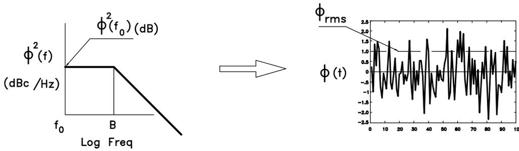
*Figure 38. PLL with Integrated VCO Phase Noise & Jitter*
