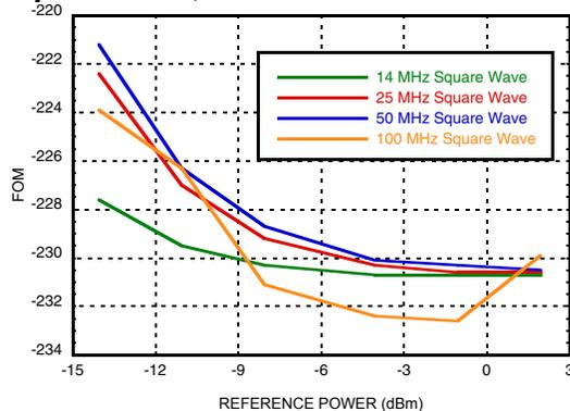
**Figure 12. Reference Input Sensitivity Sinusoidal Wave, 50 Ω<sup>[3]</sup>**
