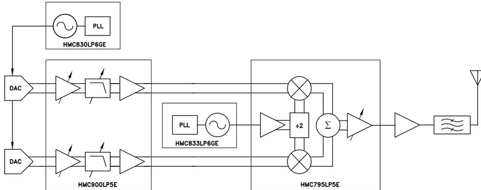
Figure 23. HMC833LP6GE in a typical transmit chain
