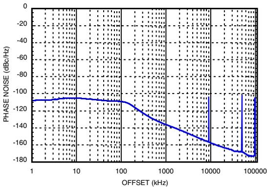
**Figure 18. Worst Spur, Fixed 50 MHz Reference, Output Freq. = 2000.1 MHz<sup>[10]</sup>**
