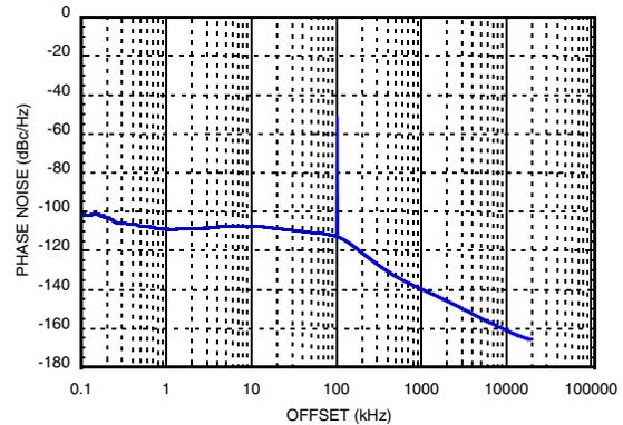
[4] Fractional Mode B, 50 MHz PD frequency, 74 kHz Loop Filter BW
