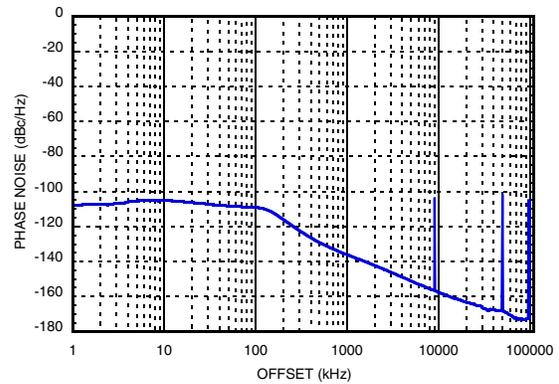
**Figure 17. Fractional-N Exact Frequency Mode OFF Performance at 2591 MHz<sup>[9]</sup>**
